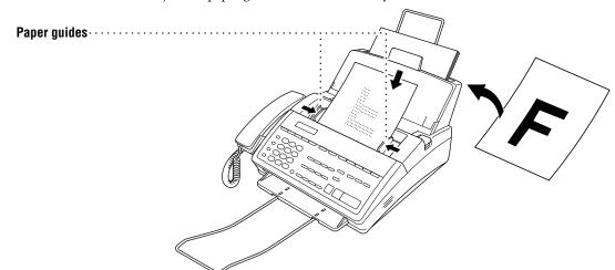
■ The automatic document feeder (ADF) can hold up to 20 pages, feeding each one individually through the FAX/MFC. Use standard (20 lb.) paper when using the ADF; if you're using heavier paper, feed each sheet individually to prevent paper jams.
