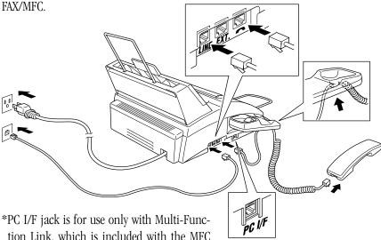
tion Link, which is included with the MFC 1870MC and MFC 1970MC, or with the optional software. If you have not purchased the *optional* Multi-Function Link (also called "Missing Link") for your FAX 1570MC, then ignore this jack.
