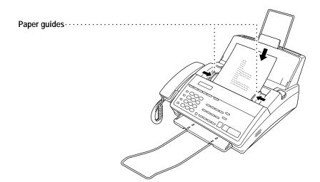
■ The automatic document feeder (**ADF**) can hold up to 20 pages, feeding each one individually through the fax machine. Use standard (20 lb.) paper when using the ADF; if you're using heavier paper, feed each sheet individually to prevent paper jams.
