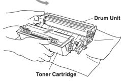
7 Clean the primary corona wire inside the drum unit by gently sliding the blue tab from right to left several times. Return the blue tab to the Home position before reinstalling the drum unit assembly.
