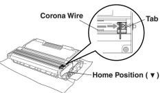
Reinstall the drum unit and close the front cover.
