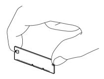
■ Make sure the memory board is securely seated on the main controller board.
