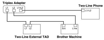
You can keep two-line telephones on other wall outlets as always. There are two ways to add a two-line telephone to the fax machine's wall outlet. You can plug the telephone line cord from the two-line telephone into the L1+L2 jack of the triplex adapter. Or, you can plug the two-line telephone into the TEL jack of the two-line TAD.
