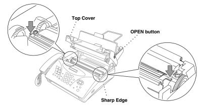
**3** Pull the jammed paper toward the back from the paper tray and remove it. If you can't, pull the jammed paper toward the front and remove it. If you cannot see any jammed paper, take out the ribbon cassette and check underneath. Remove any jammed paper.
