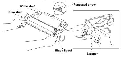
**4** Turn the black spool on the right clockwise to tighten the ribbon.
