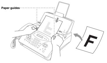
■ The ADF can hold up to 20 pages (17lb -20 lb), feeding each one individually through the fax machine. Use standard (17 lb -24 lb) paper when using the ADF; if you're using heavier paper, feed each sheet individually to prevent paper jams.
