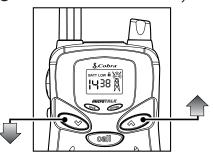
2 Select any of the 14 channels by pushing the channel up or down buttons.
