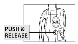
1 Push and release P LIGHT/MAX RANGE button to illuminate display for ten seconds.
