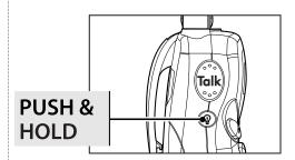
• Push and hold • LIGHT/MAX RANGE button to allow all signals to enter.
