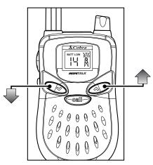
2 Select any of the 14 channels by pushing the channel up or down buttons.
