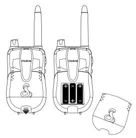
• Pull lock tab down to remove battery cover.
