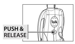
1 Push and release P LIGHT/MAX RANGE button to illuminate display for ten seconds.
