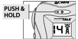
1 Push and hold the POWER button for 2 seconds. An audible "tone" will indicate the unit is on.
