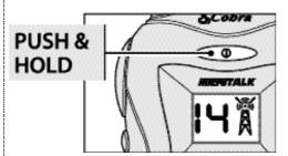
**1** Turn on your microTALK® 2-way radio. An audible "tone" will indicate the unit is on.
