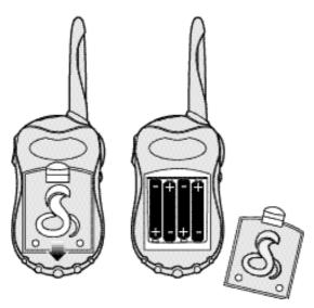
**1** Pull lock tab down to remove battery cover.
