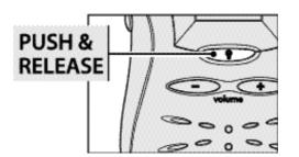
• Push and release LIGHT/MAX RANGE button to illuminate display for ten seconds.
