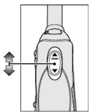
2 Select any of the 14 channels by moving the channel button up or down.
