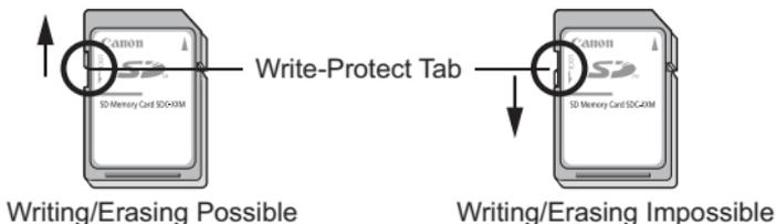
Ensure that the memory card is correctly oriented before inserting it in the camera. It may damage the camera if inserted backward by mistake.
