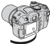
Fold the LCD monitor back against the camera body until it clicks into place.
