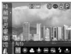
The white balance cannot be adjusted when the photo effect is set to (Sepia) or (B/W) (p. 94).
