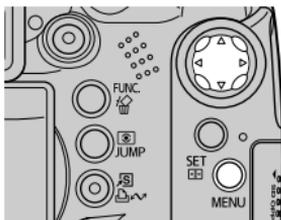
**3** Use the ▲ or ▼ button on the omni selector to select [Format], then press the SET button.
