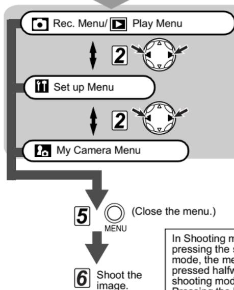
In Shooting mode, the menu can be closed by pressing the shutter button halfway. (In Playback mode, the menu closes when the shutter button is pressed halfway and the camera switches to shooting mode.) Pressing the Movie button returns to shooting mode and also closes the menu.
