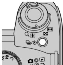
**2** Press the shutter button halfway to lock the focus.
