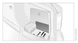
The onboard tool kit is stored in a compartment on the right-hand side of the cargo bay. Remove the cover.
