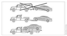
Have the BMW transported with a tow truck with a so-called lift bar or on a flat bed.
