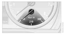
During standard operation, the engine oil temperature is between approx. 160 °F /70 °C and approx. 340 °F/170 °C. If the engine oil temperature is too high, a message will appear on the Control Display.
