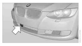
The sensor's ability to detect vehicles ahead may be restricted as a result of heavy rain, dirt, snow or ice. If necessary, clean the radar sensor located in the front bumper, see arrow. Be sure to use particular care when removing any layers of snow or ice from the sensor.
