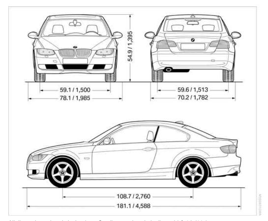
All dimensions given in inches/mm. Smallest turning circle diam.: 36 ft 1 in/11.0 m 335i: height approx. 4 ft 6 in/1,375 mm
