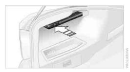
The warning triangle is located on the left-hand side of the cargo bay. Press the tab to take it out.
