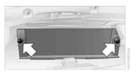
Open the cover in the glove compartment and remove it.
