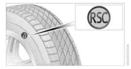
The symbol identifying Run-Flat Tires is a circle with the letters RSC on the sidewall. Run-Flat Tires comprise a conditionally self-
