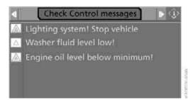
Some Check Control messages remain visible until the malfunction in question has been rectified. They cannot be hidden. If several malfunctions occur at the same time, the Check Control messages are displayed in succession.
