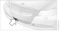
The sensor's ability to detect vehicles ahead may be restricted as a result of heavy rain, dirt, snow or ice. If necessary, clean the radar sensor located in the front bumper, see arrow. Be sure to use particular care when removing any layers of snow or ice from the sensor.
