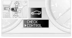
Lightly push button 1 in the turn indicator stalk repeatedly up or down until the appropriate symbol appears in the display, accompanied by the words "CHECK CON-TROL".
