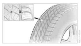
Wear indicators in the base of the tread groove are distributed around the tire's circumference; the letters TWI, Tread Wear Indicator, on the tire's sidewalls identify tires that incorporate these wear indicators. Once the tire tread has worn down to the wear indicators, the tire has worn to a depth of 1/16 in/1.6 mm.
