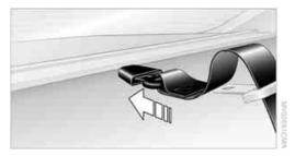
Push the corresponding head restraint down as far as it will go, refer to page 41.  To release the rear seat back, pull the corresponding lever in the luggage compartment.
