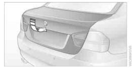
Press the button, see arrow, or press the button on the remote control for approx. 1 second. The luggage compartment lid will open slightly. It can now be swung upwards.
