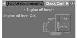
Select "Engine oil level" and press the controller. The oil level is displayed.
