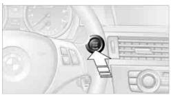
Each time the start/stop button is pressed, radio readiness or the ignition is switched on or off.
