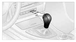
A lock prevents you from inadvertently engaging selector lever positions R and P. To cancel the lock, press the button on the front of the selector lever knob, refer to arrow.
