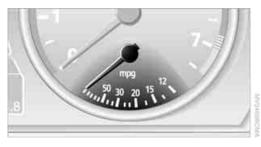
Displays the current fuel consumption. This allows you to see whether your current driving style is conducive to fuel economy with minimum exhaust emissions.
