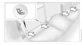
The anchorage points for the LATCH childrestraint fixing system are located underneath the identifying symbols.
