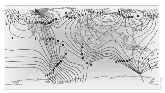
To set a compass zone, press the adjustment button on the bottom of the interior rearview mirror with a pointed object, such as a pen, for approx. 3-4 seconds. The number of the compass zone set is shown in the display.
