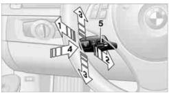
Press the lever upward or downward, arrow 3. The displays in the speedometer disappear. In addition, the system is automatically deactivated:
