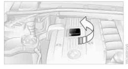
Do not add the maximum amount of 1.1 US quarts/1 liter of engine oil until a corresponding message is shown on the Control Display.
