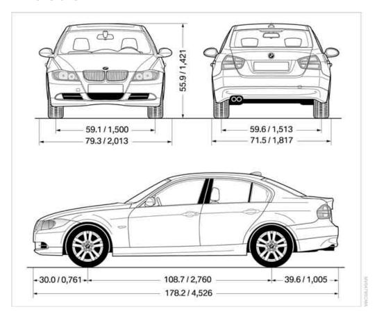
All dimensions given in inches/mm. Smallest turning circle diam.: 36 ft 1 in/11.0 m
