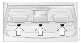
If you use a child-restraint system with a tether strap, three additional tether anchorage points have been provided, refer to the arrows in the illustration. Depending on the location selected for seating in the rear passenger area, attach the tether strap to the corresponding anchorage point to secure the child-restraint system, as shown in the illustration below.
