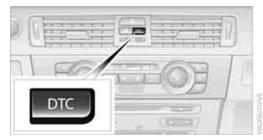
Briefly press the button; the DTC indicator lamps in the instrument cluster come on.
