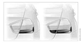
The brake lamps light up in two stages, depending on how sharply you apply the brakes.
