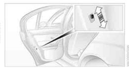
Slide down the safety lever on the rear doors: The door can now be opened from the outside only.
