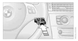
Insert the remote control all the way into the ianition lock.
