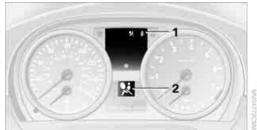
Indicator and warning lamps can light up in both the indicator area 1 and the display 2 in various combinations and colors.
