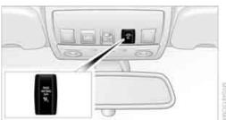
The indicator lamp located above the rearview mirror indicates whether the front passenger airbag system is active or not active/OFF.
