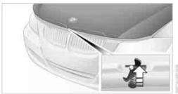
In order to avoid damage, make sure that the wiper arms are against the windshield before you open the hood.◀
