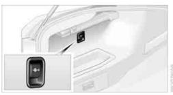
To gain access to the power socket: Open the cap.
