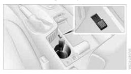
The storage compartment in the center armrest can be ventilated: push the switch to position 1.
