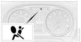
When the remote control is inserted into the ignition lock or the car is radio-ready, refer to page 49, the warning lamp comes on briefly to indicate that the entire airbag system and the belt tensioners are operational.
