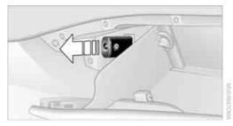
Only insert the flashlight back into the socket when it is switched off, as otherwise there is a risk of damage. ◀
