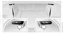
The unlocked rear seat back moves forward slightly. Fold the seat back forward by the head restraint.
