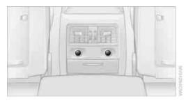
To gain access to the power socket: Remove the corresponding cover.
