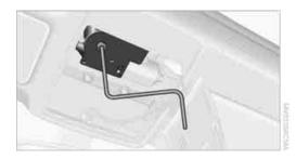
Reattach the cover for the interior lamps and install the cover panel.
