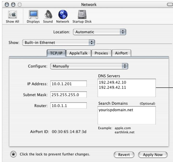
When you configure Ethernet clients manually for a base station that provides NAT over Ethernet, you can use IP addresses in the range 10.0.1.201 to 10.0.1.254.
