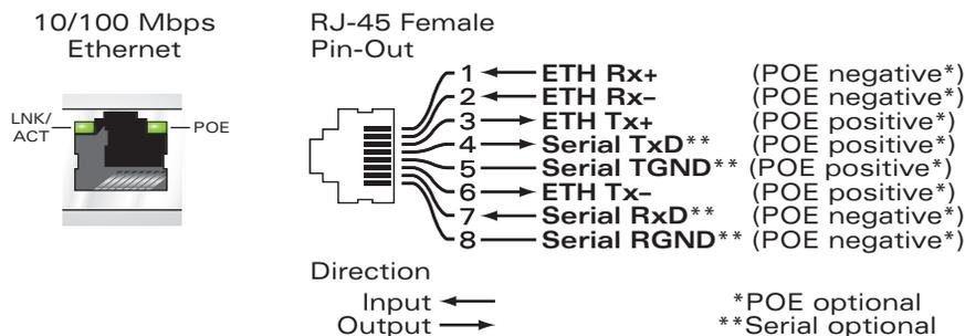
**FIGURE B-2 FE Network Port Pin-outs**
