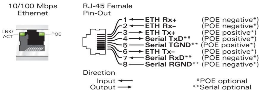
**FIGURE B-2 FE Network Port Pin-outs**
