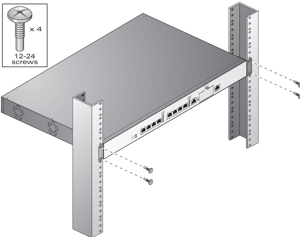
**FIGURE 2-3** Mounting the Alcatel Wireless LAN Switch
