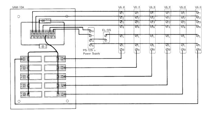
NOTE: If EL-9S electric door release is not installed, you do not need to wire L, L terminals on each VA-K station.
