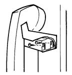
Install the handset cradle with provided screws as shown at left.
