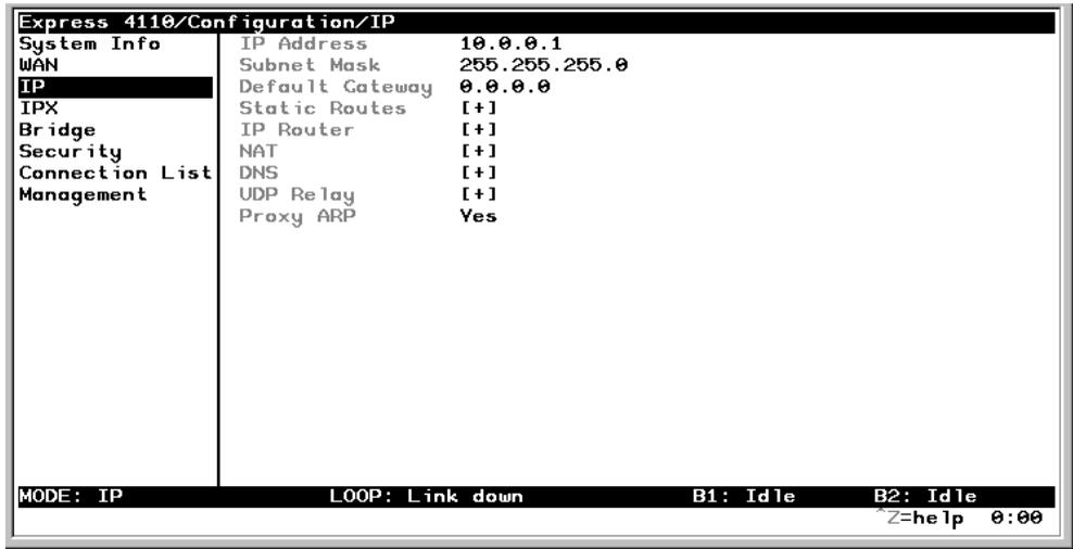
**Figure 3-4. Configuration/IP Screen**
