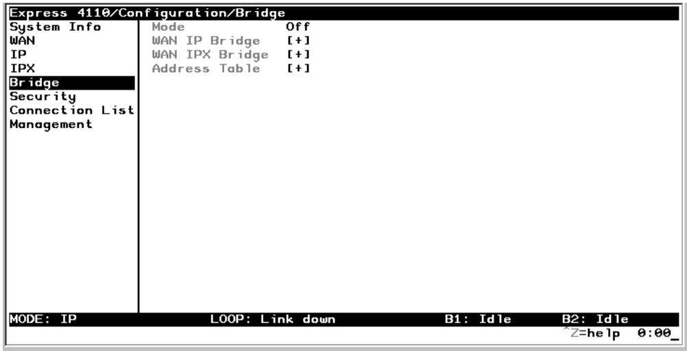
Figure 3-6. Configuration/Bridge Screen
