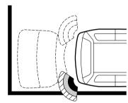
In this example, the corner sensor detects the side wall.
