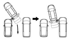
The sensors may not work if the ambient air temperature is below -4°F (-20°C) or above 122°F (50°C).
