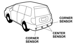
The sensors are designed to give you an audible signal when the rear bumper of your vehicle is approaching an obstacle.
