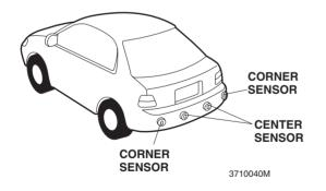
The sensors are designed to give you an audible signal when the rear bumper of your vehicle is approaching an obstacle.
