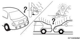
The sensors may not work if the obstacle is an odd shape or made of material that does not reflect ultrasonic waves.
