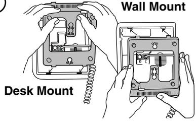
Attach the wedge-shaped base in desk mount or wall mount position†.
