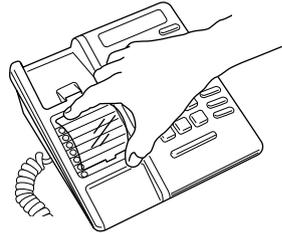
Attach the receiver card and lens (shiny-side down) after recording numbers for quick reference.
