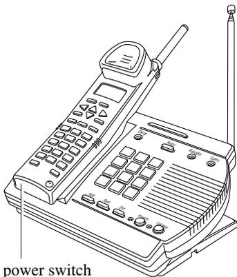
1. Leave the phone on the base as shown, with the charge light on and the **handset power switch off**.
