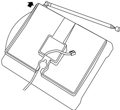
3. Plug the line cord into the wall jack. Line up the screws on the wall mount plate with the openings in the stand and slide the phone down until the mounting screws hold firmly.
