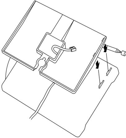
2. Slide the stand into the locked position, as shown below.
