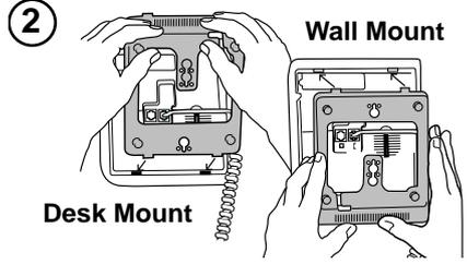
Attach the wedge-shaped base in desk mount or wall mount position†.
