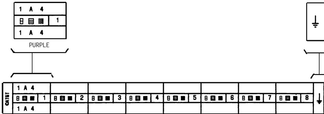
Figure 3-37. Example of Port Label for 16-Port Analog Line Circuit Pack
