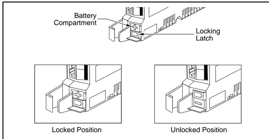
**Figure 6-1. Battery Compartment PARTNER Endeavor processor module**
