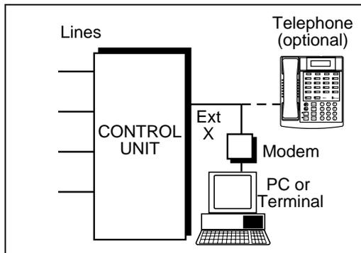
**Figure 4-9. Stand-Alone Modem for Placing Calls Only**
