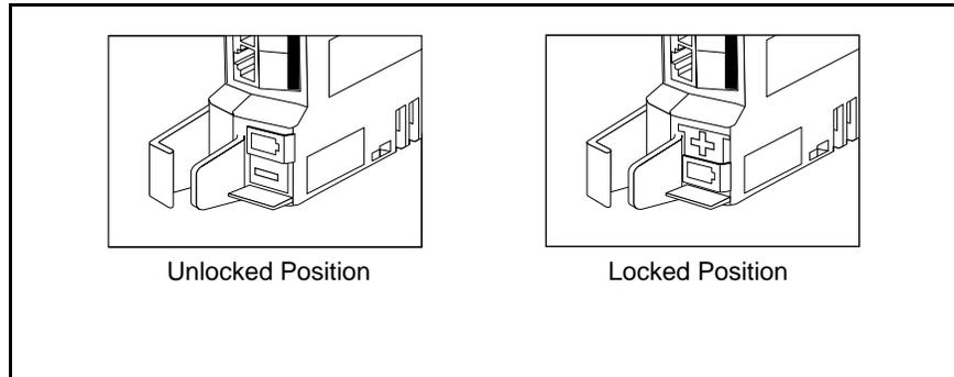
**Figure 6-5. Battery Assembly in Unlocked and Locked Position**
