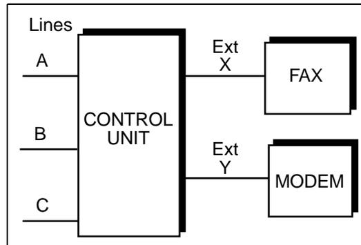
**Figure 4-11. Night Service with Fax Machine and Modem**
