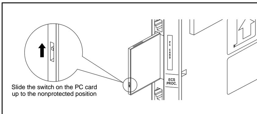
**Figure 6-6. Write-Protect Tab on a Backup/Restore PC Card**
