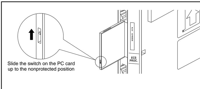
**Figure 6-7. Write-Protect Tab on a Backup/Restore PC Card**
