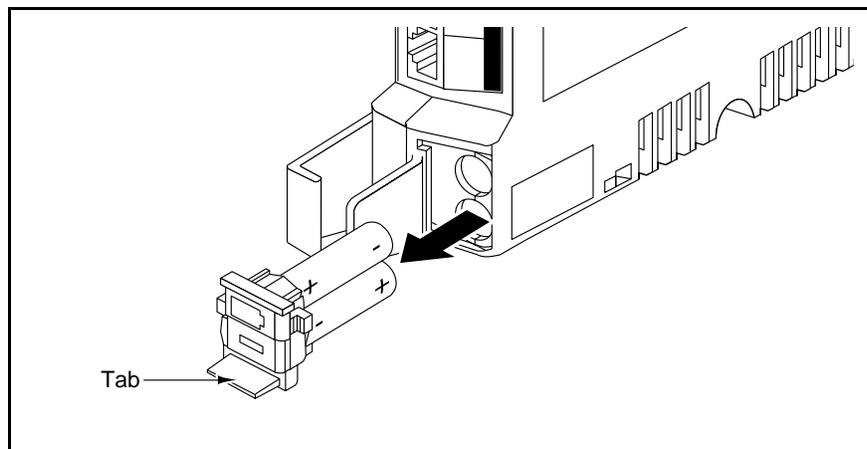
**Figure 6-2. Removing the Battery Assembly**
