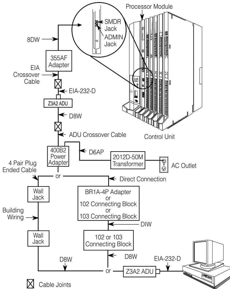
Figure 2-2. Direct Local Connection, PC More Than 50 ft. Away
