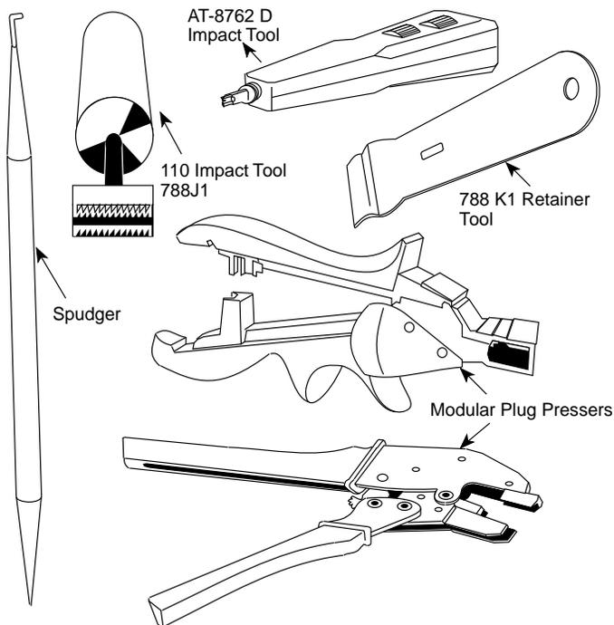
**Figure 4-3. RJ21X Wiring Field Tools**
