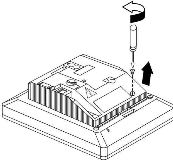
**Figure 3-5. Releasing the Module Cover Screw**
