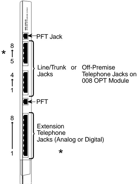
Figure 2-12. Line/Trunk and Telephone Jack Locations on Each Module
