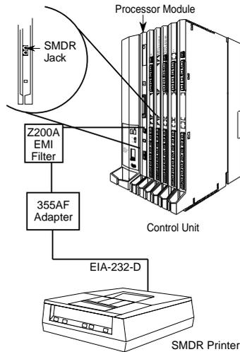
**Figure 5-5. Connecting a Printer Within 50 ft. (15.2 m)**
