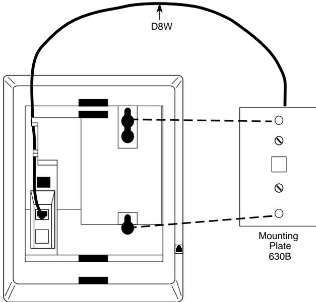
**Figure 3-38. Routing the Cord Through the Backplate**
