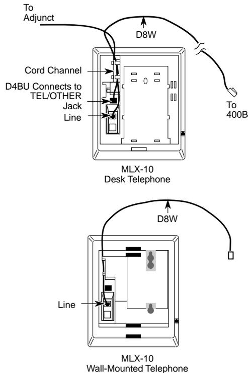
**Figure 3-20. Routing the Cord(s) Through the Cord Channel**
