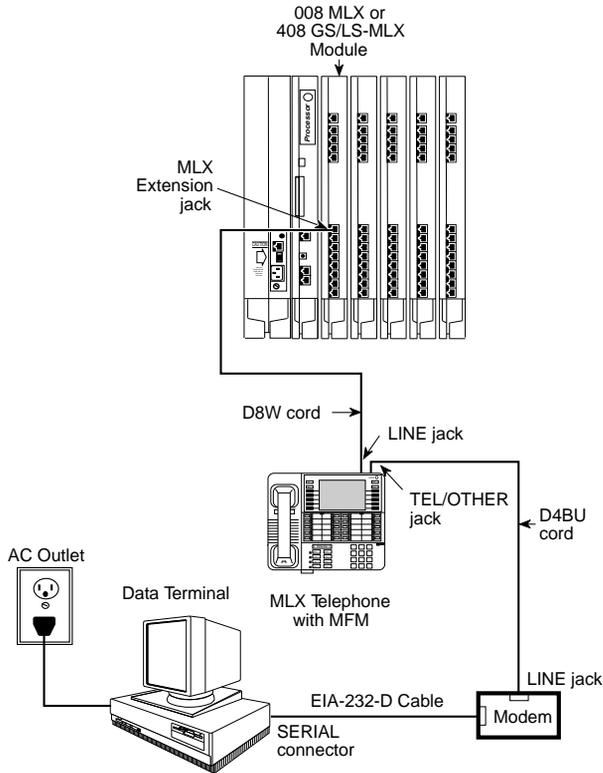
Figure 6-3. Modem Data and MLX Voice Equipment Configuration
