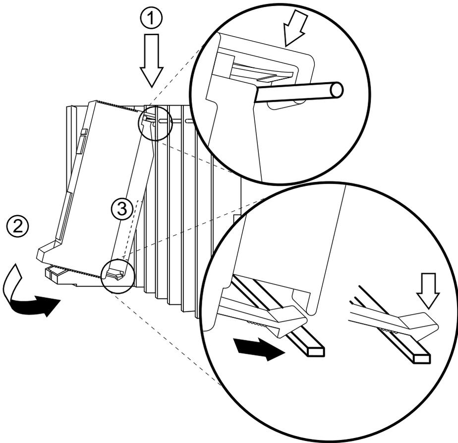
Figure 2-10. Installing the Processor into the Carrier
