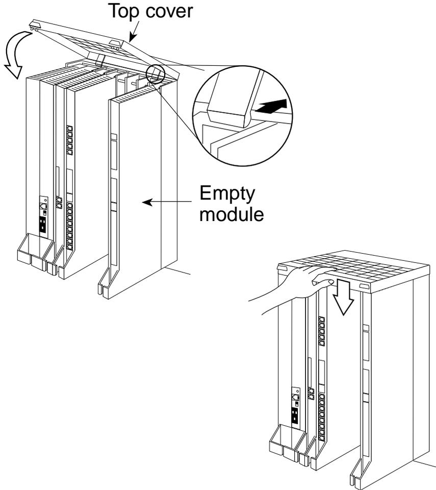
Figure 7-2. Installing the Control Unit Top Cover
