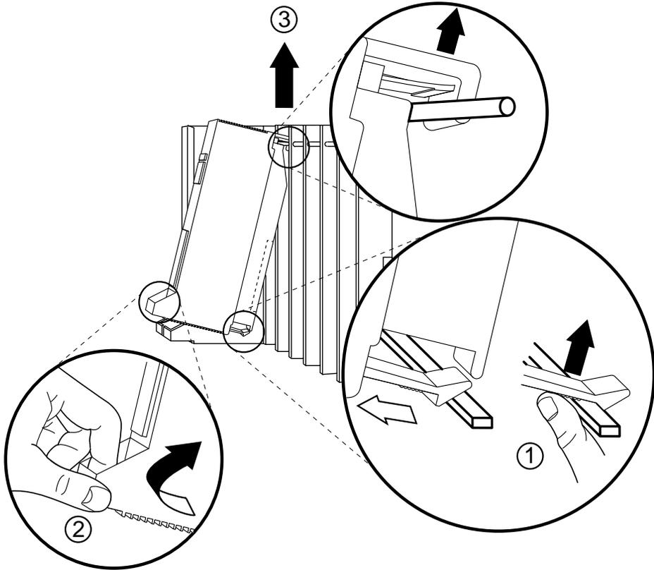
Figure 2-13. Removing Modules from the Carrier
