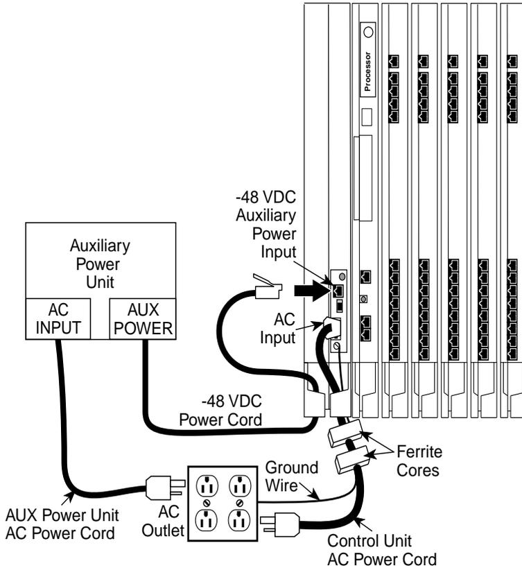
Figure 2-8. Installing an Auxiliary Power Unit
