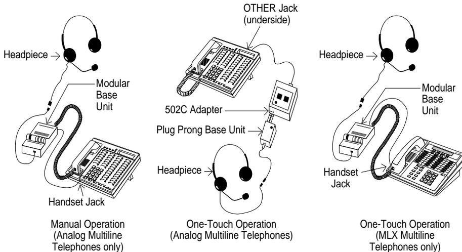
**Figure 3-21. Manual and One-Touch Headset Operation**
