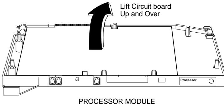
**Figure 9-6. Removing the Processor Module Circuit Board**
