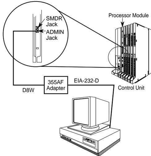
**Figure 5-1. Connecting a PC Within 50 ft. (15.2 m)**
