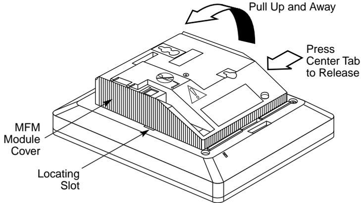
**Figure 3-6. Releasing the Module Cover**
