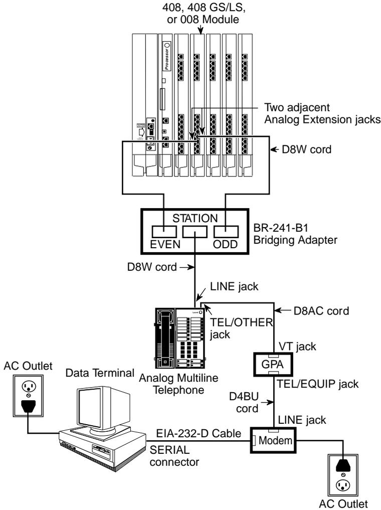
Figure 6-1. Analog Voice and Modem Data Equipment Configuration
