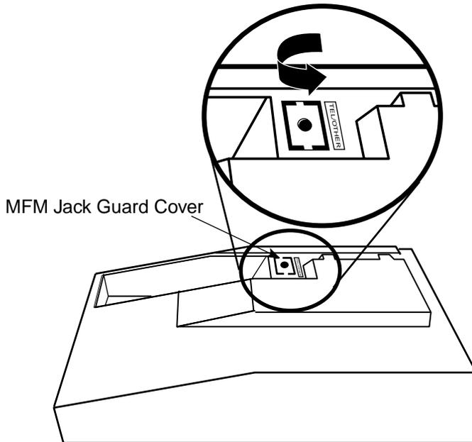
**Figure 3-11. Removing the Jack Guard**
