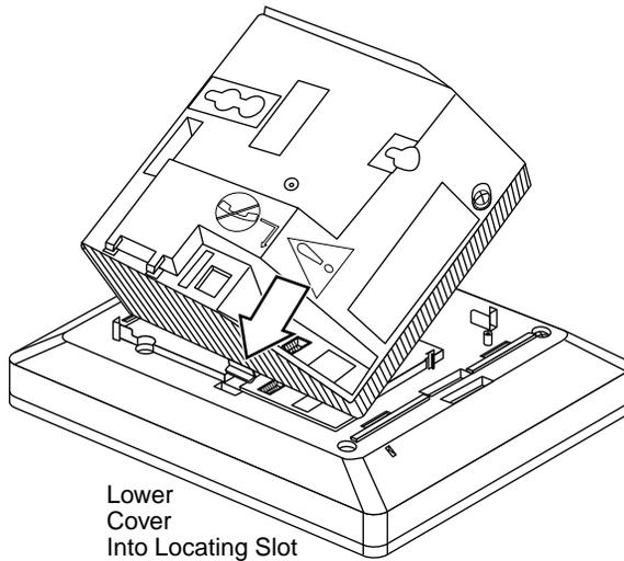
**Figure 3-12. Placing the Module Cover into the Locating Slot**
