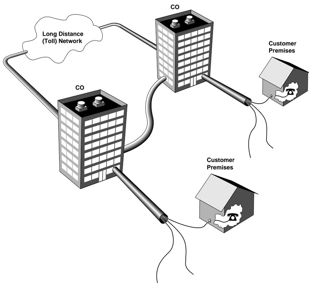
Figure 2-2. The Telephone Network
