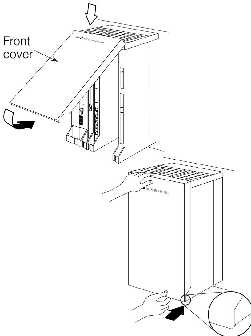
Figure E-3. Installing the Front Cover
