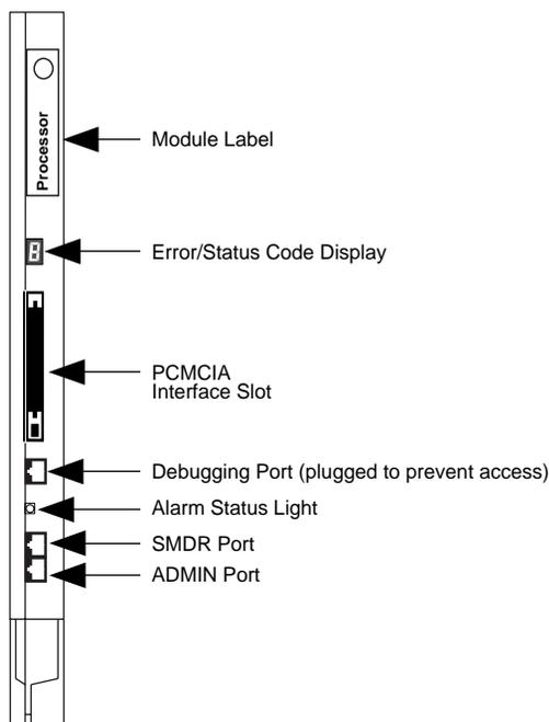
**Figure 3-1. Processor Module**
