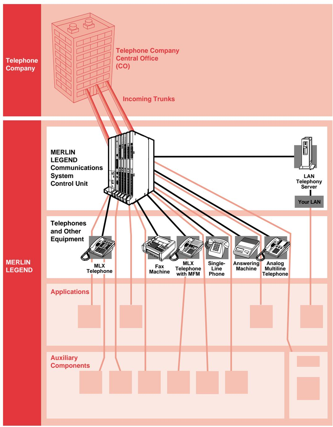
Figure 2-7. System Components
