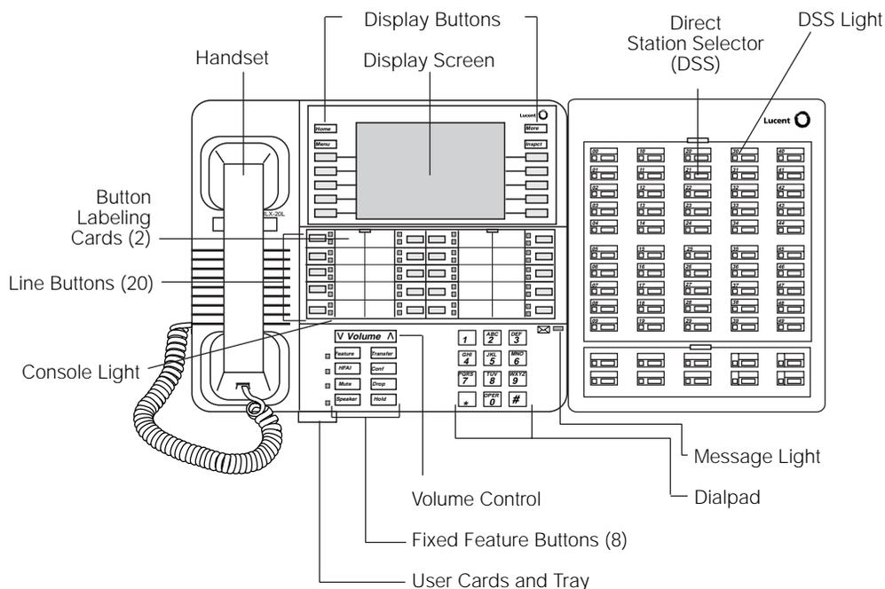
**Figure 6-7. MLX-20L Telephone with Direct Station Selector (DSS)**
