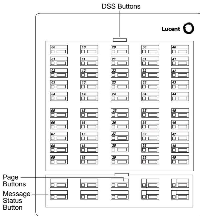
**Figure 3-10. Direct Station Selector**
