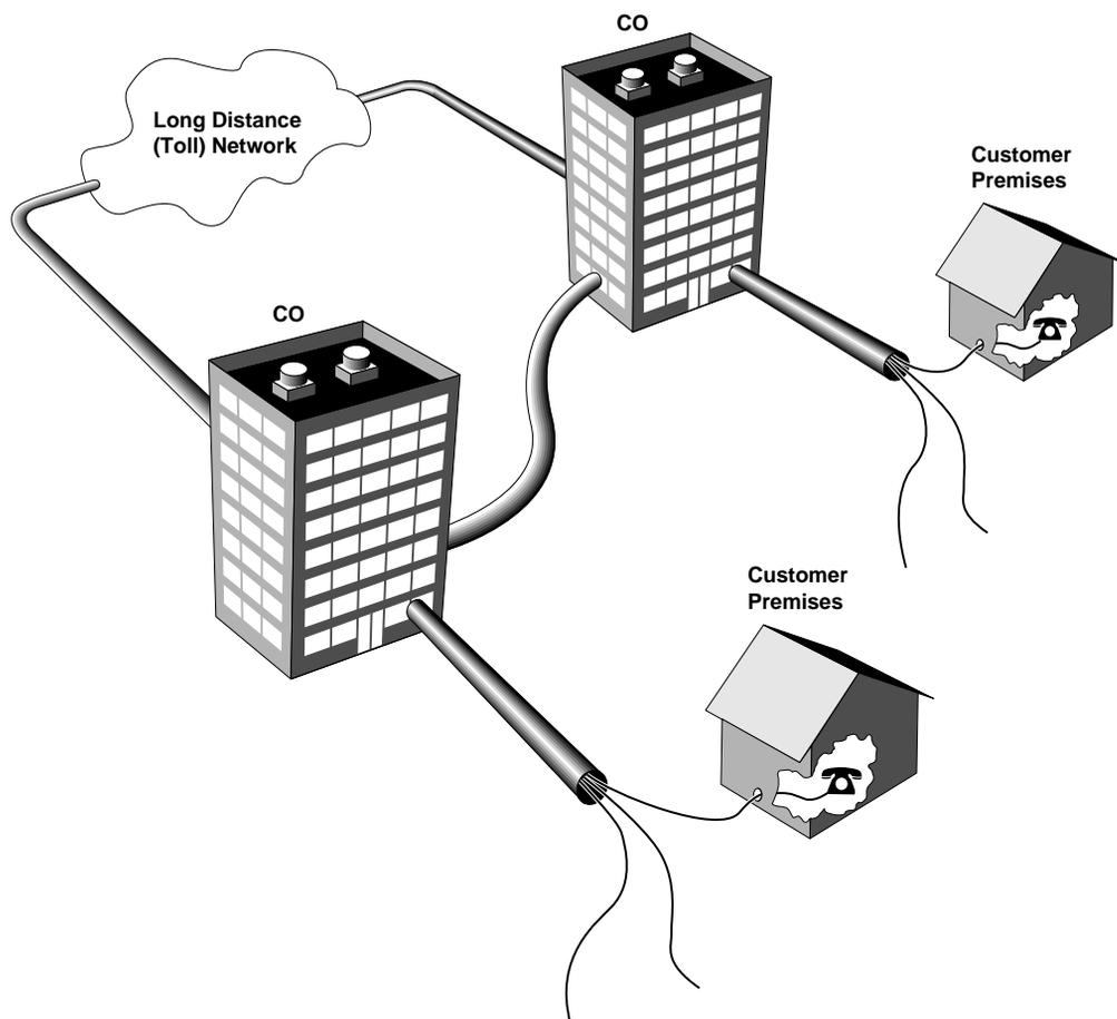
Figure 2-2. The Telephone Network
