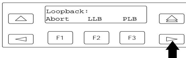
Figure 4-13. ACCULINK 3150 CSU DTE Loopback Command 3
