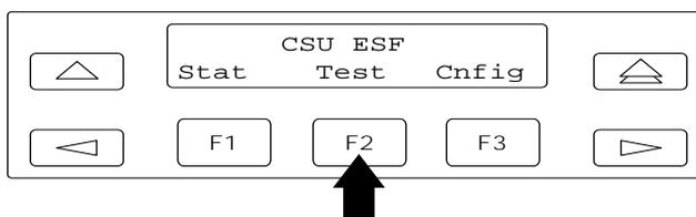
Figure 4-11. ACCULINK 3150 CSU DTE Loopback Command 1
