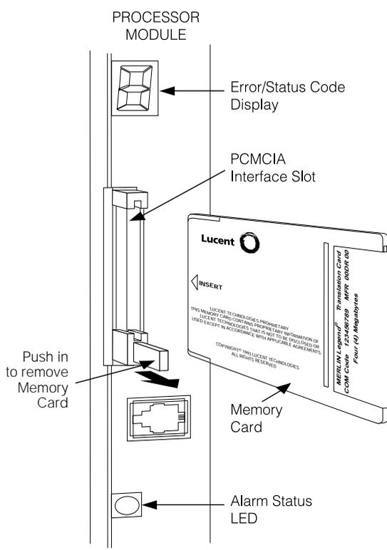
Figure D-2. Inserting the Memory Card
