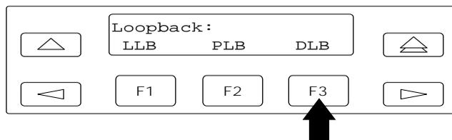
**Figure 4-14. ACCULINK 3150 CSU DTE Loopback Command 4**
