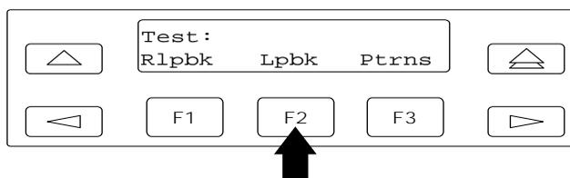
Figure 4-12. ACCULINK 3150 CSU DTE Loopback Command 2
