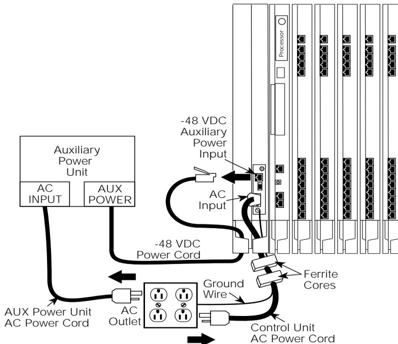
Figure 4-3. Replacing an Auxiliary Power Supply
