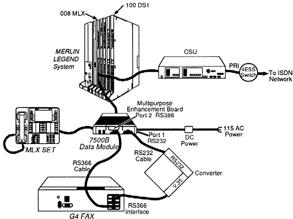
**Figure 5-3. RS-232 to V.35 Interface Conversion**
