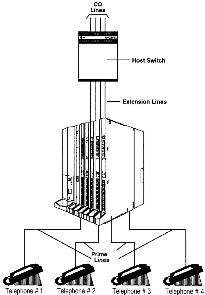
**Figure 1-6. Behind Switch Mode**
