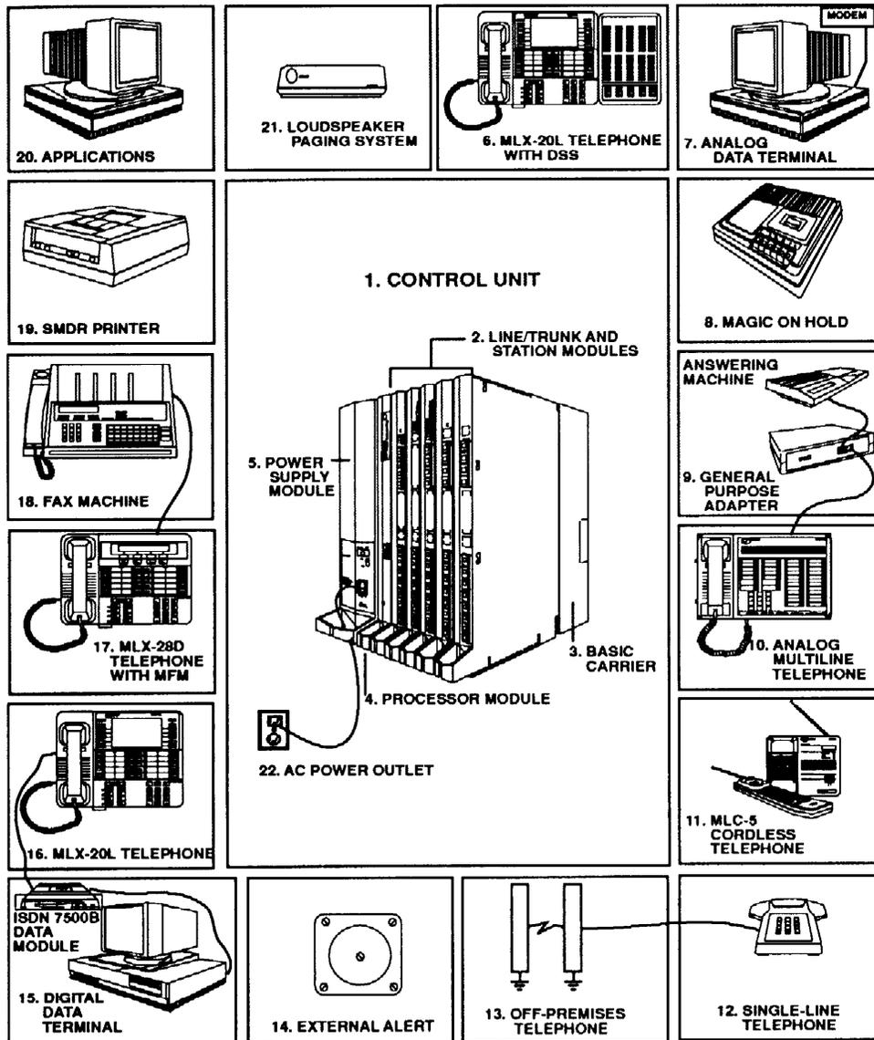
Figure 1-1. System Components
