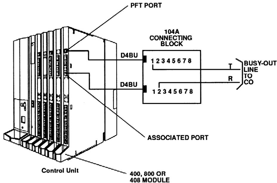
Figure 2-25. Power Failure DID Busy-Out Connections
