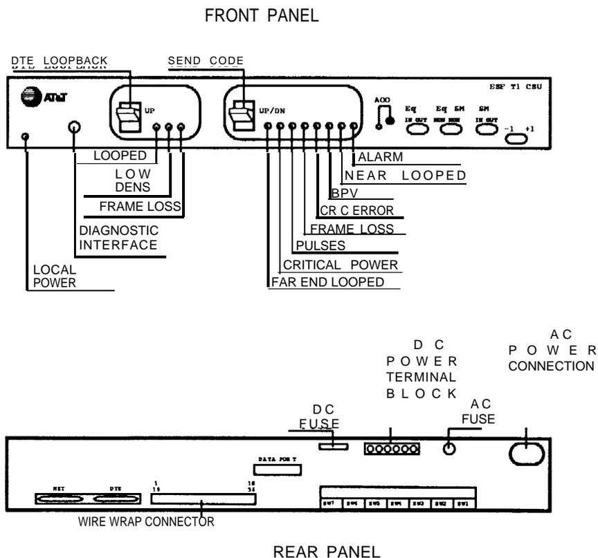
Figure 2-12. ESF T1 Channel Service Unit Connections
