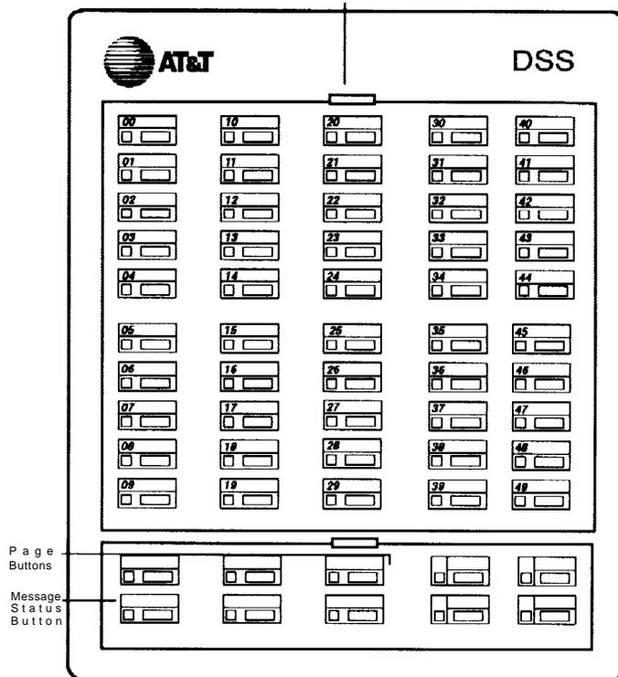
**Figure 2-10. Direct Station Selector**
