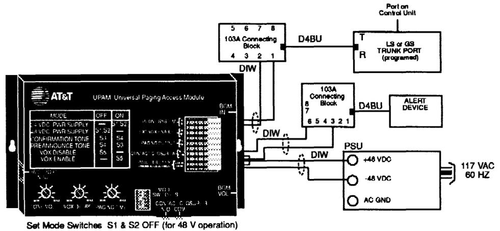
Figure 2-23. Trouble Alarm Connections
