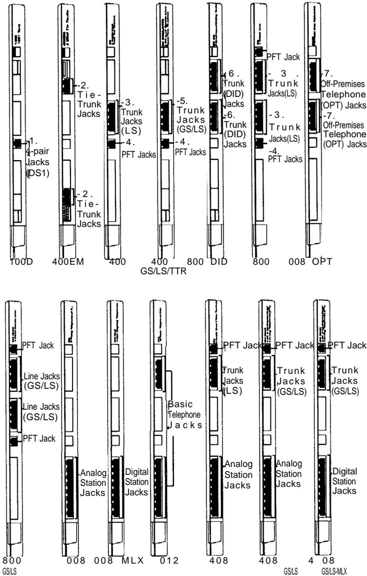
Figure 2-4. Line/Trunk and Station Modules
