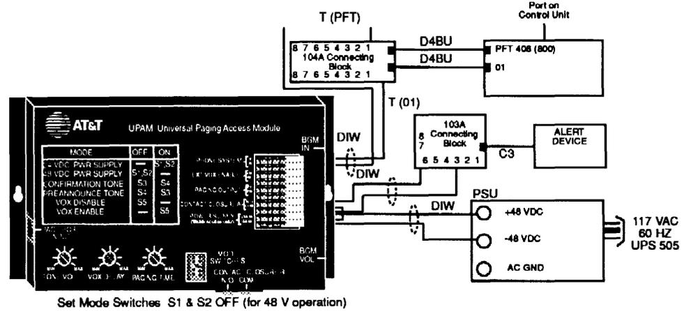
Figure 2-24. Power Failure Alarm Connections
