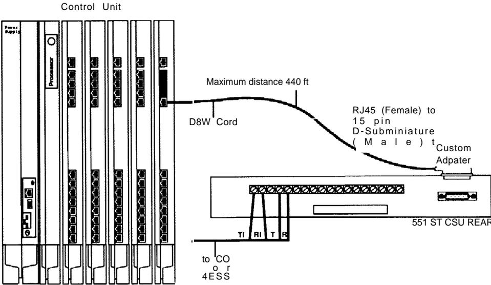
Figure 2-11. 551 T1 L1 Channel Service Unit Connections
