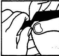
3. Insert the label strips into the slots on the console. Slot numbers on the black tabs indicate the correct slot for the strip. Slot 1 is on the far left\* slot 7 is on the far right.
