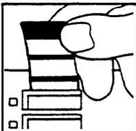
\* Note the control unit jack numbers (A0-B2) printed on the line button labels. Label each button with the telephone number of the outside line that is plugged into the control unit jack whose number is printed on the button label.
