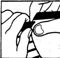
3. Insert the label strips into the console. Slot numbers on the black tabs indicate the correct slot for the strip. Slot 1 is on the far left; slot 4 on the far right.
