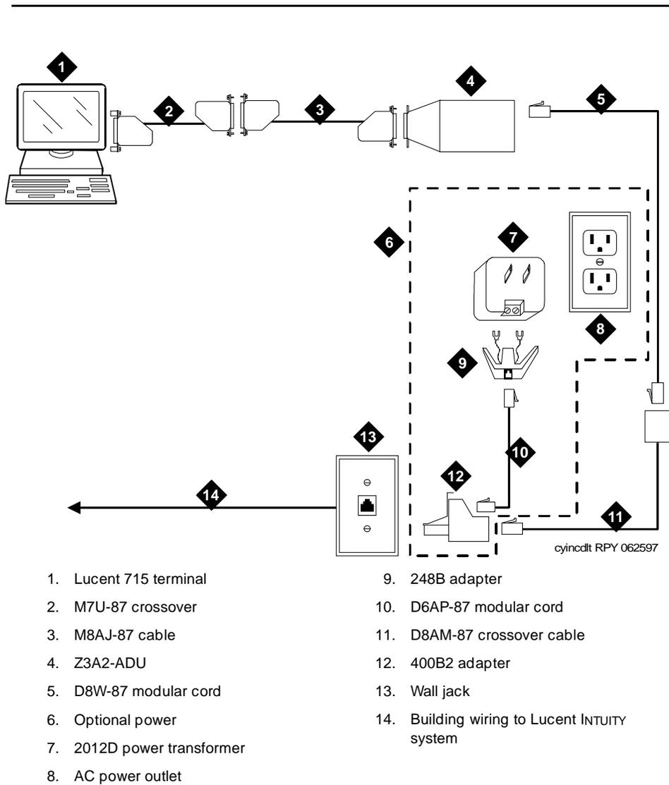
**Figure 4-8. Connecting a Dedicated Line Terminal Beyond 50 Feet (15 Meters): Terminal End**
