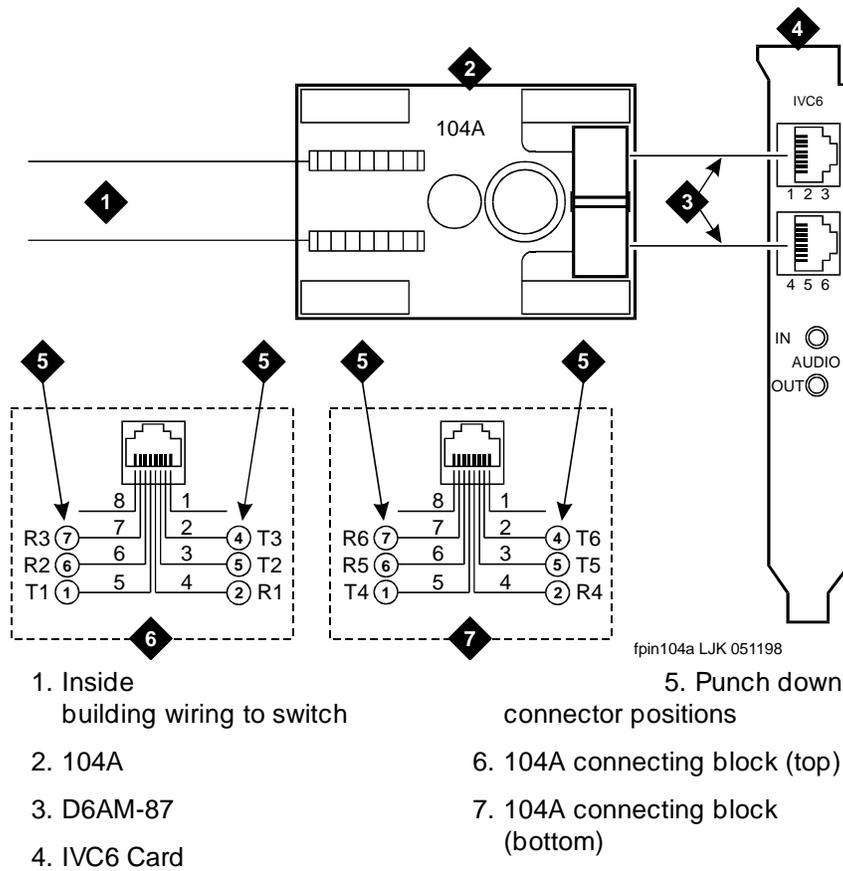
Figure 4-2. Connecting IVC6 Cards Using 104A Connecting Blocks
