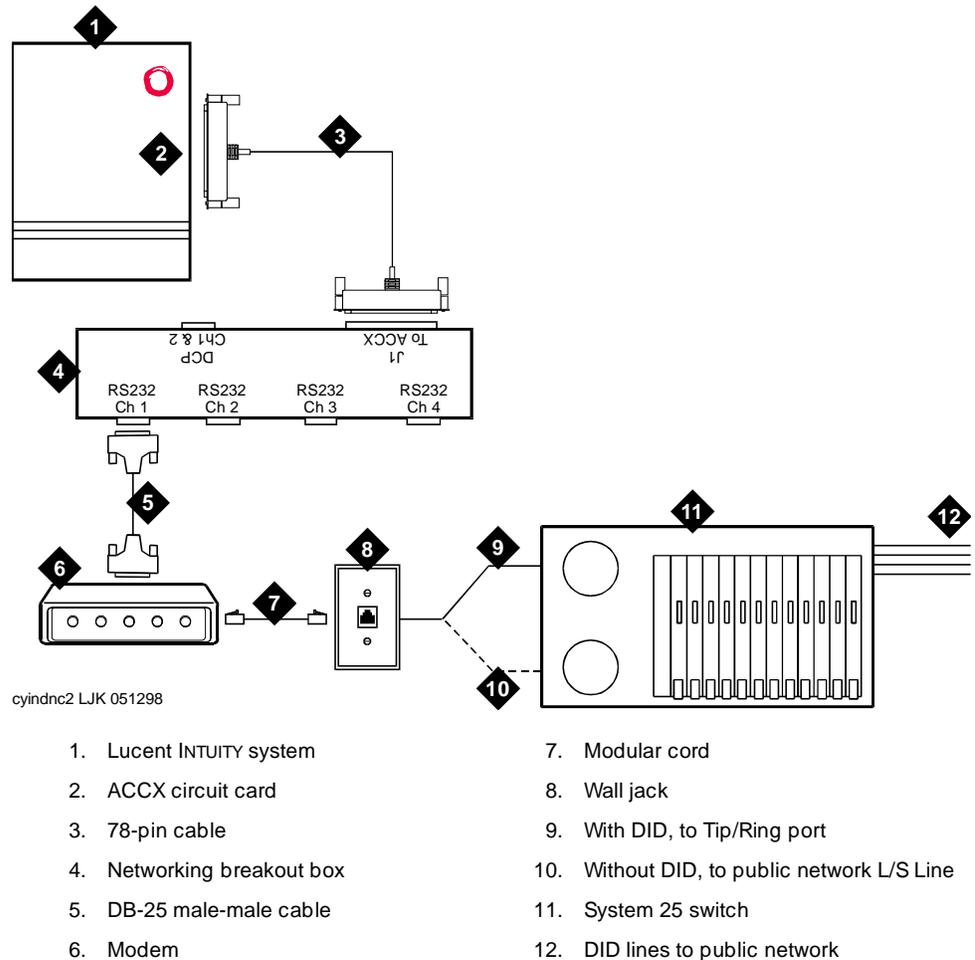
Figure 4-6. Digital Networking Connections
