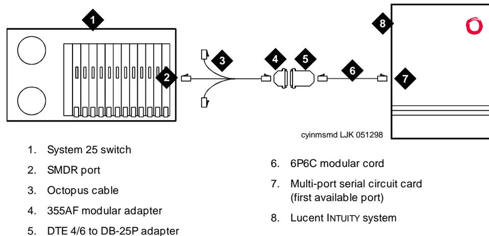
Figure 4-4. Connecting SMDR Ports Within 50 Feet, and Same Power Outlet (Multi-Port Serial Circuit Card)
