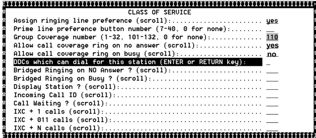
Figure 5-12. Class of Service Window; Assigning Station Coverage
