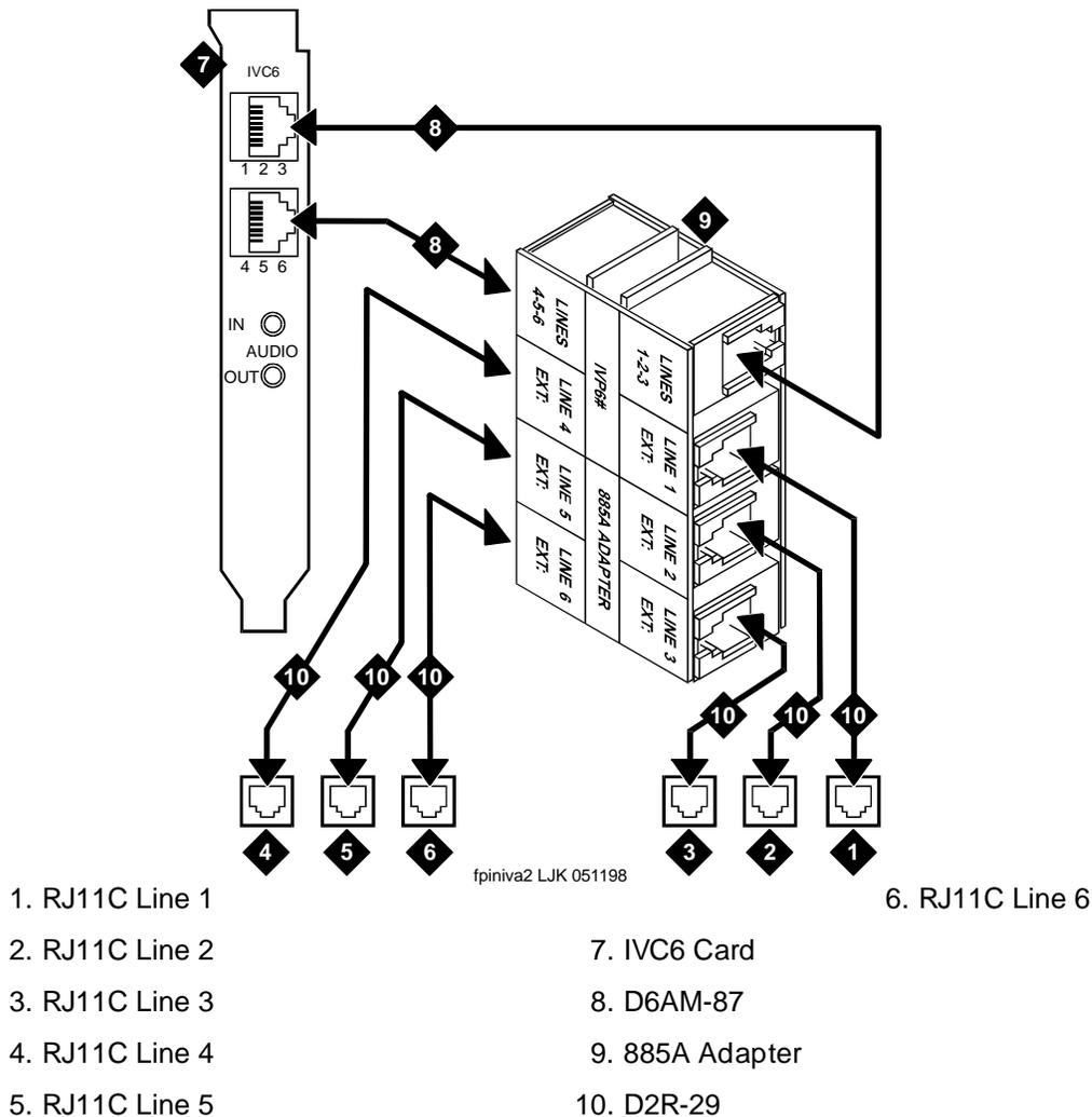
Figure 4-1. Connecting IVC6 Cards Using an 885A Adapter
