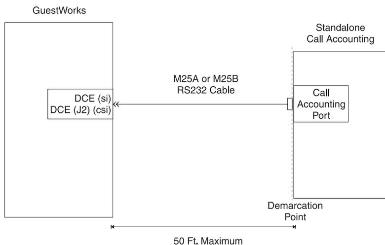
**Figure 13. Switch-to-Call Accounting Link (Stand-alone Call Accounting System)**
