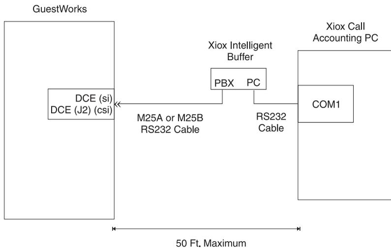
**Figure 12. Switch-to-Call Accounting Link (Xiox Call Accounting System)**
