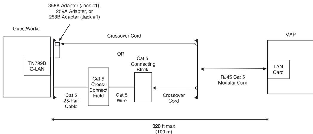
Figure 3. Switch-to-INTUITY Admin Link (TCP/IP) with Crossover Cord
