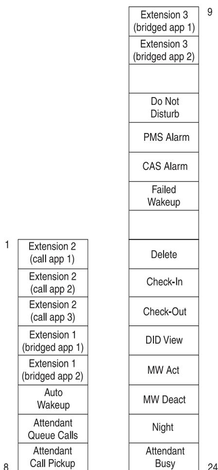
Figure 26. First Backup Telephone Button Layout (Model 6424)
