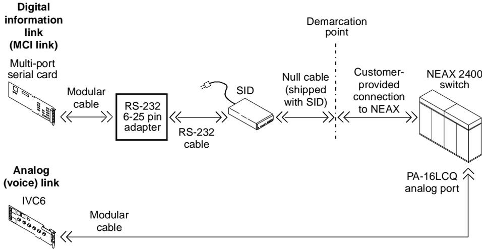
Figure 4-2. NEAX Connections to the INTUITY System
