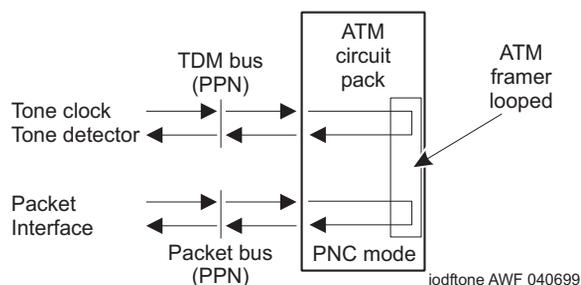
**Figure 3-5. ATM Board Framer Looparound Test (#1260)**
