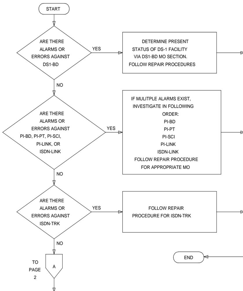
Figure 1-16. Processing of ISDN-PRI Problems (Page 1 of 2)
