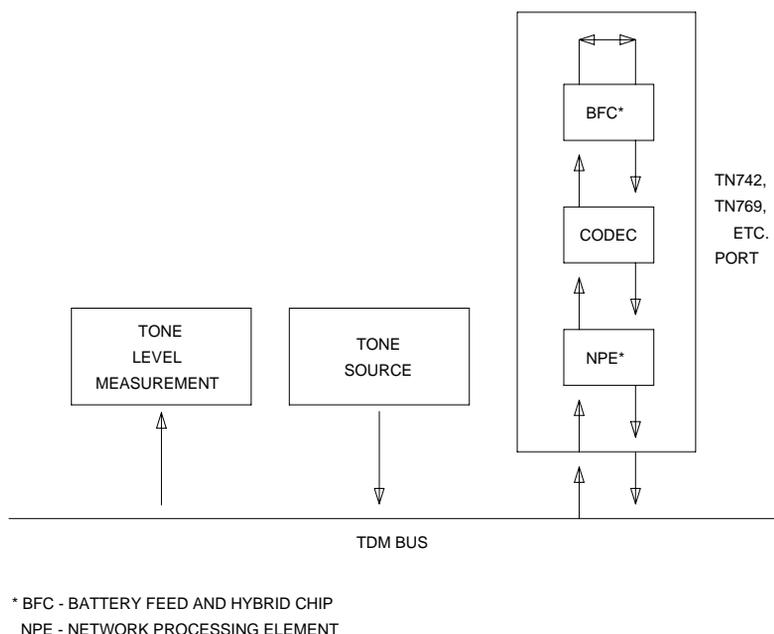
Figure 3-1. Analog Loop Around and Conference Test
