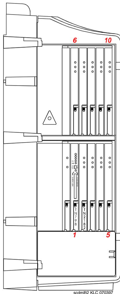
**Figure 1-1. Compact Modular Cabinet (CMC) slot configuration**
