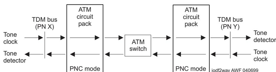
**Figure 3-3. Expansion Interface 2-Way Transmit Test #241**
