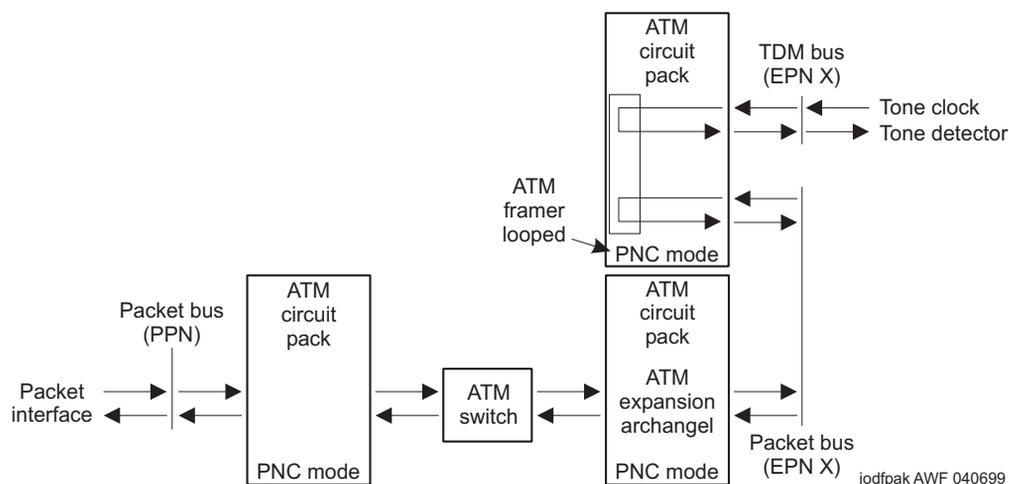
**Figure 3-6. ATM Board Framer Looparound Test (#1260)
