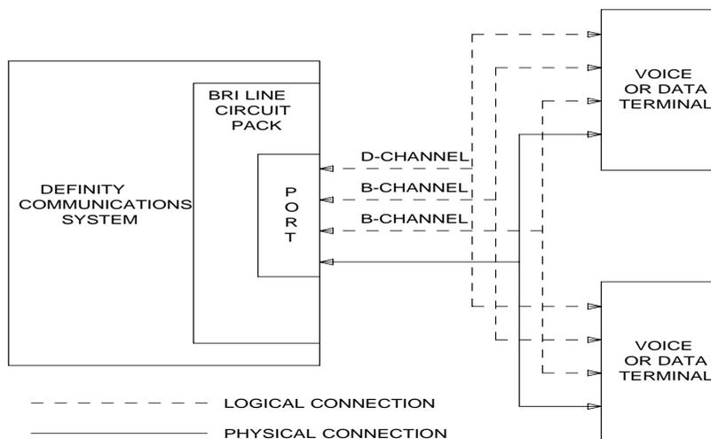
**Figure 3-11. ISDN-BRI Port Interactions****Hardware Error Log Entries and Test to Clear Values****Table 3-117. ISDN-BRI Port Error Log Entries**
