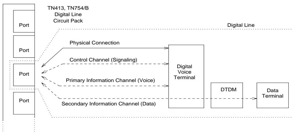
Figure 3-17. Digital Line Connectivity
