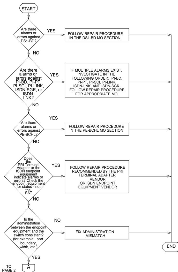
Figure 1-18. Processing of PRI Endpoint Problems (Page 1 of 2)
