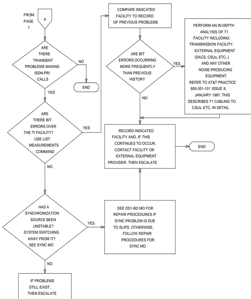
Figure 1-17. Processing of ISDN-PRI Problems (Page 2 of 2)
