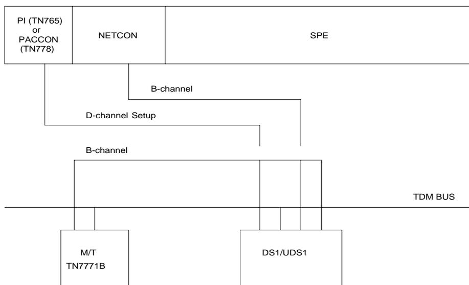
Figure 3-28. ISDN-PRI Outgoing Test Call
