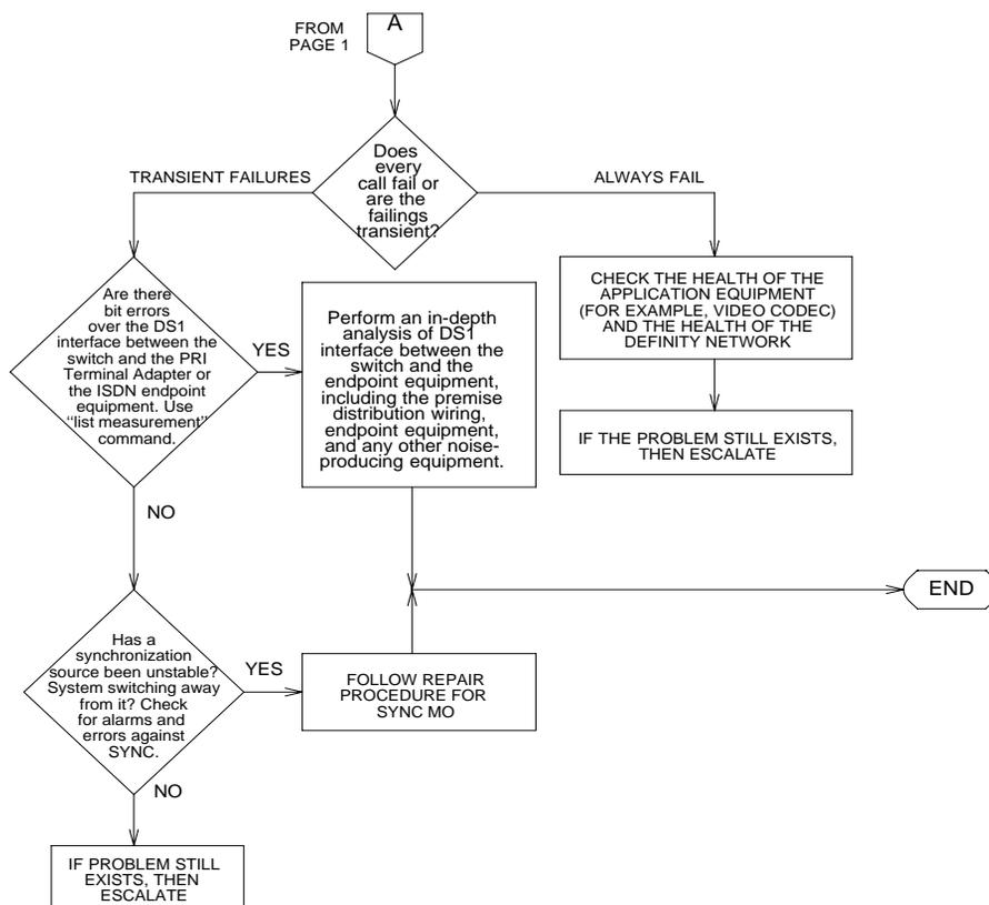
Figure 1-19. Processing of PRI Endpoint Problems (Page 2 of 2)
