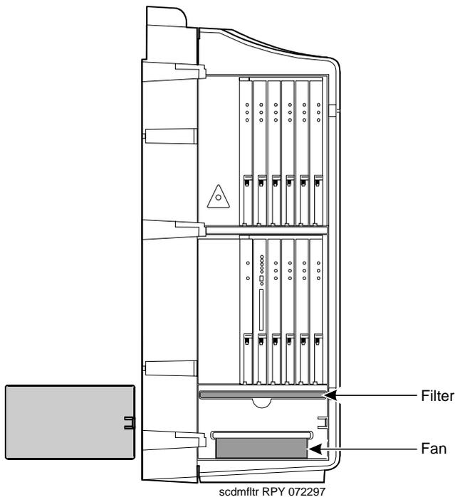
**Figure 1-3. Fan/Filter Removal**
