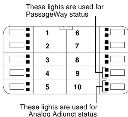
Figure 12-13. The Location of Buttons #9 and #10 on the 8411
