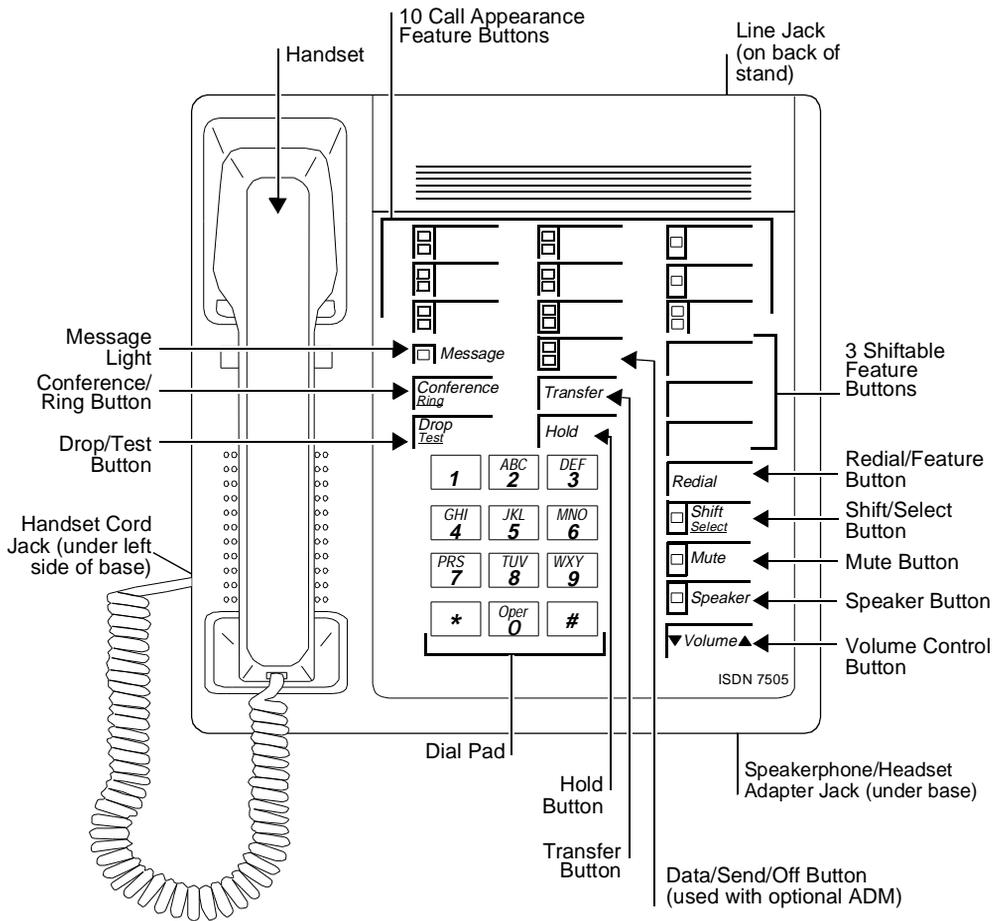
Figure 16-1. The 7505 Asynchronous Data Modular Terminal
