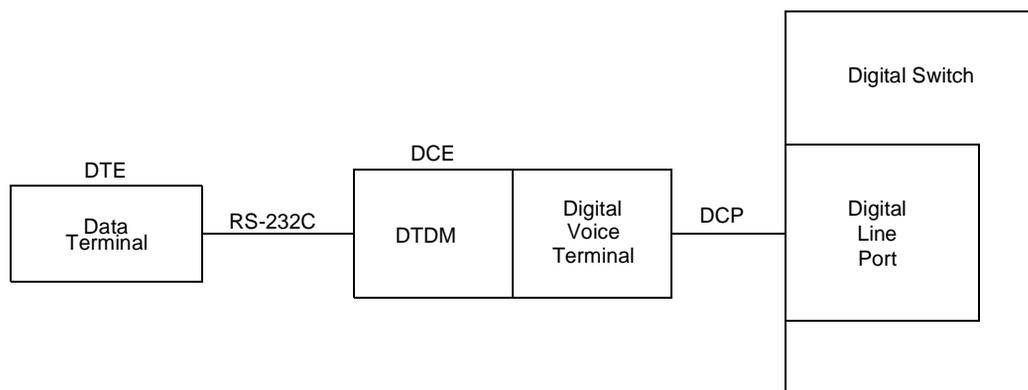
**Figure 20-11. A Block Diagram of DTDM Interfaces**
