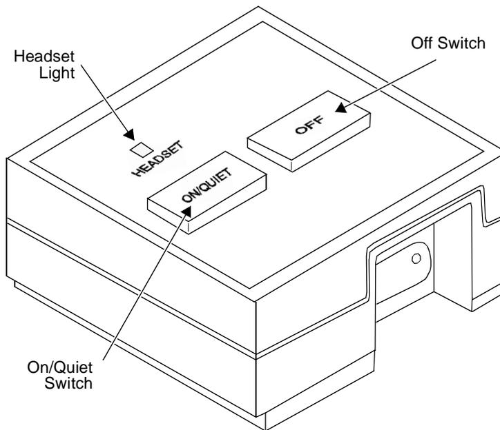
**Figure 19-6. The 500A Headset Adapter**
