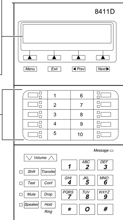
Figure 12-14. Button Numbering for Administering the 8411 Voice Terminal Connected to a System 75, a DEFINITY G1 or G3, or a DEFINITY ECS
