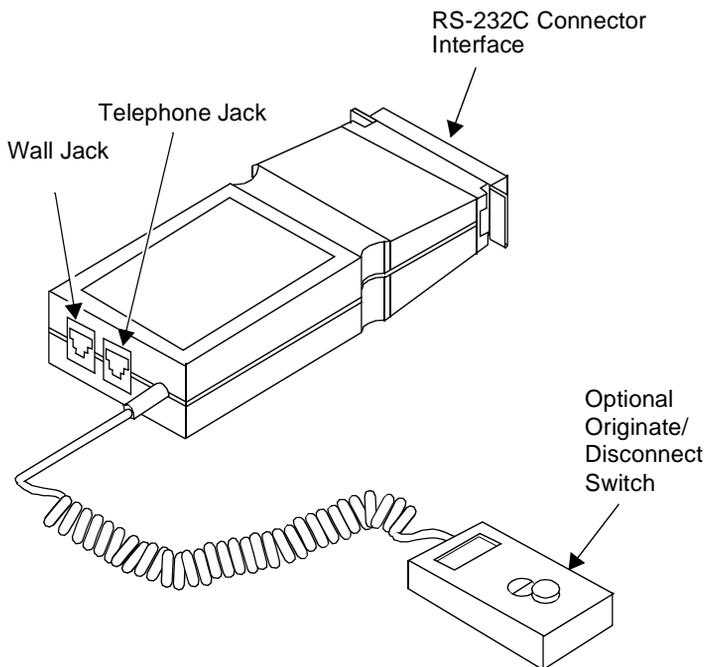
**Figure 20-25. The Z3A Asynchronous Data Unit**
