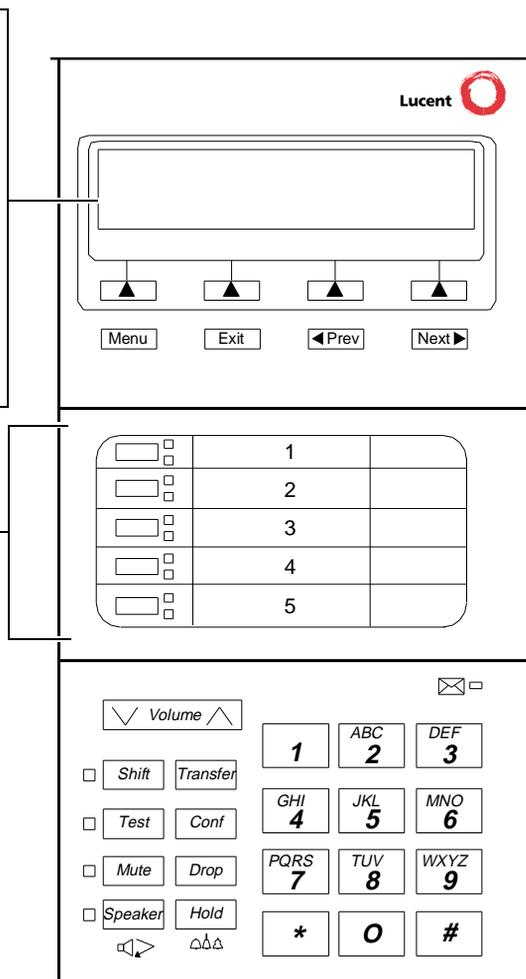
Figure 12-6. Button Numbering for Administering the 8405 Voice Terminal Connected to a System 75, a DEFINITY G1 or G3, or a DEFINITY ECS
