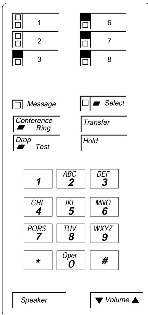
Figure 11-5. Button Numbering for Administering the 7402 Plus Voice Terminal Connected to a System 75, a DEFINITY G1 or G3, or a DEFINITY ECS
