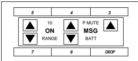
Figure 17-9. Button Numbering for an MDW 9000 Connected to a System 85 or a DEFINITY Generic 2
