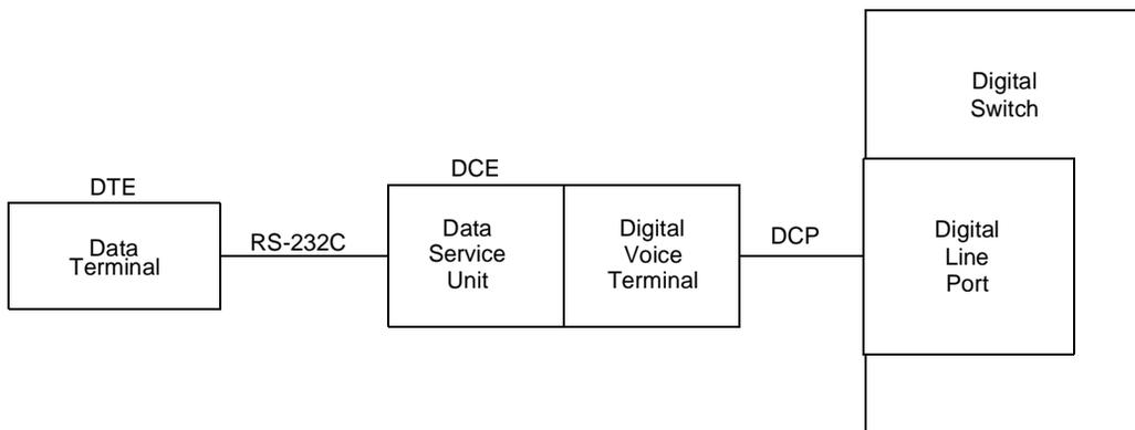
**Figure 20-13. A Block Diagram of Z702AL1 Data Service Unit Interfaces**
