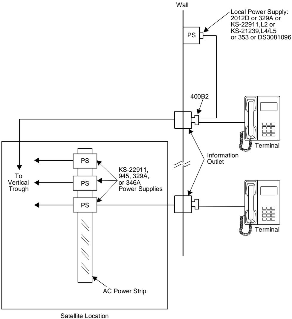
Figure 5-1. Local and Satellite Power Sources for Voice Terminals Adjuncts
