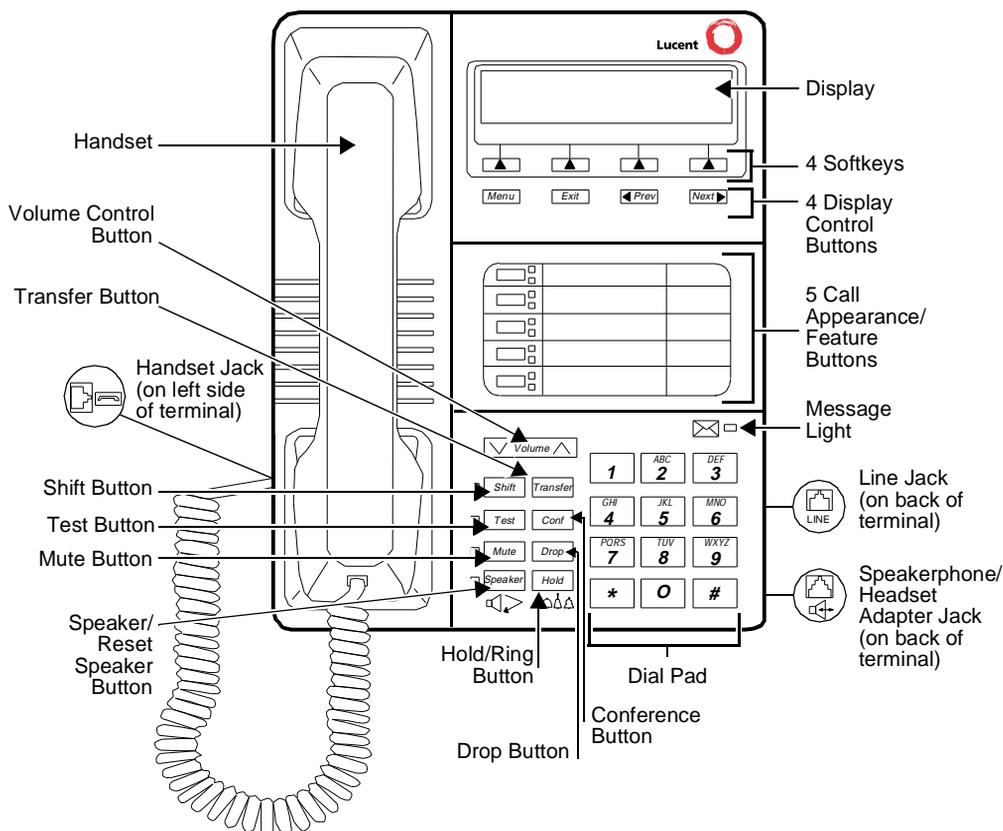
**Figure 12-5. The 8405D and 8405D Plus Voice Terminal (With Display)**
