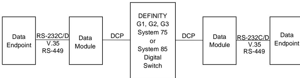
**Figure 2-3. Data Link Components**
