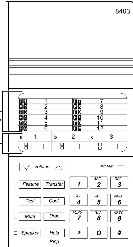
Figure 12-2. Button Numbering for Administering the 8403 Voice Terminal Connected to a System 75, DEFINITY G1 or G3, or DEFINITY ECS
