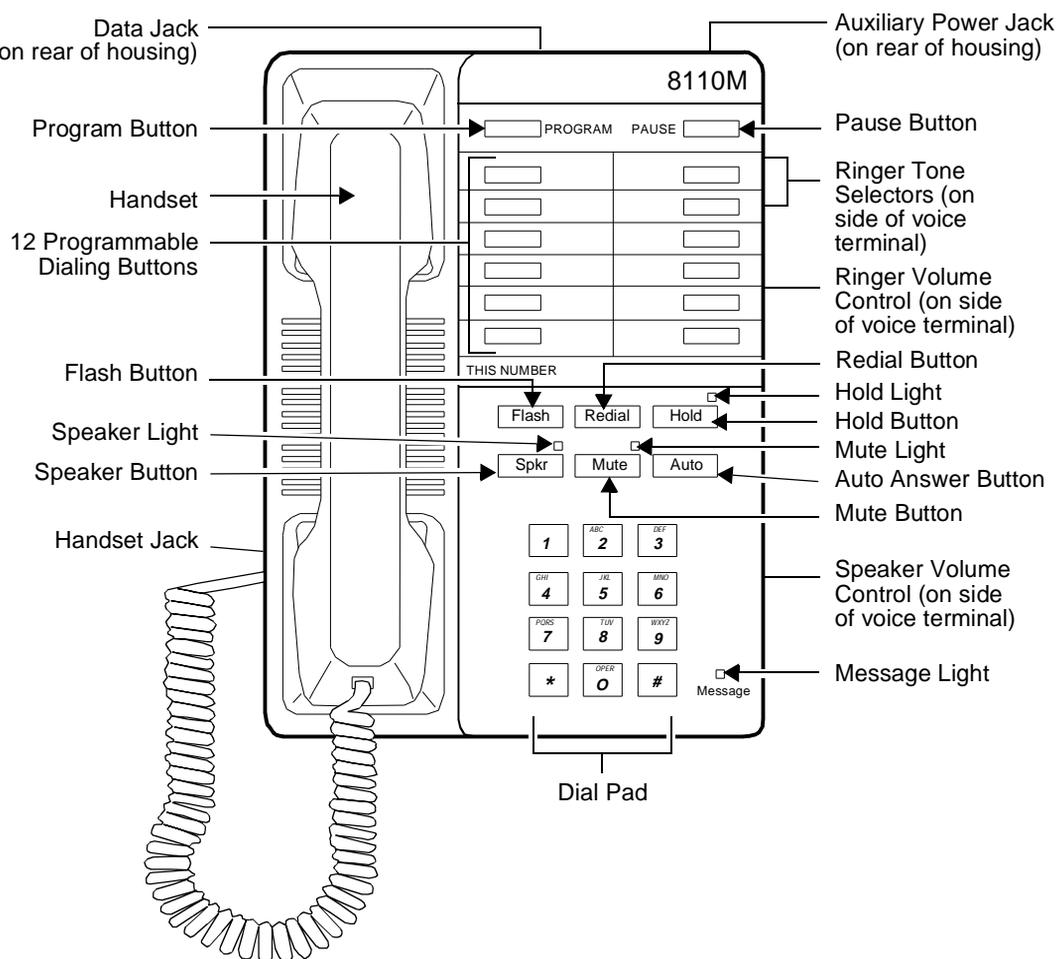
**Figure 15-4. The 8110 and 8110M Telephones (The 8110M is shown here)**
