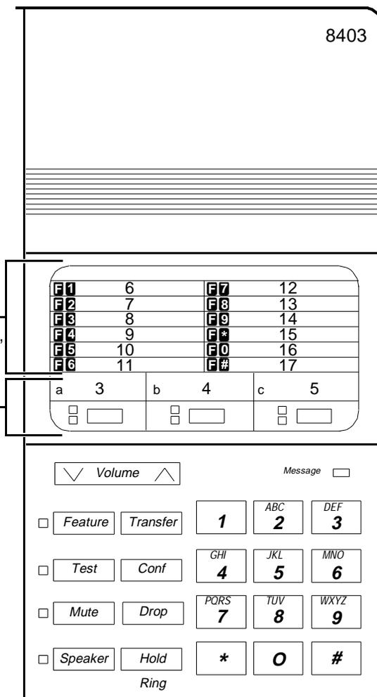
**Figure 12-3. Button Numbering for Administering the 8403 Voice Terminal Connected to a System 85 or a DEFINITY G2**
