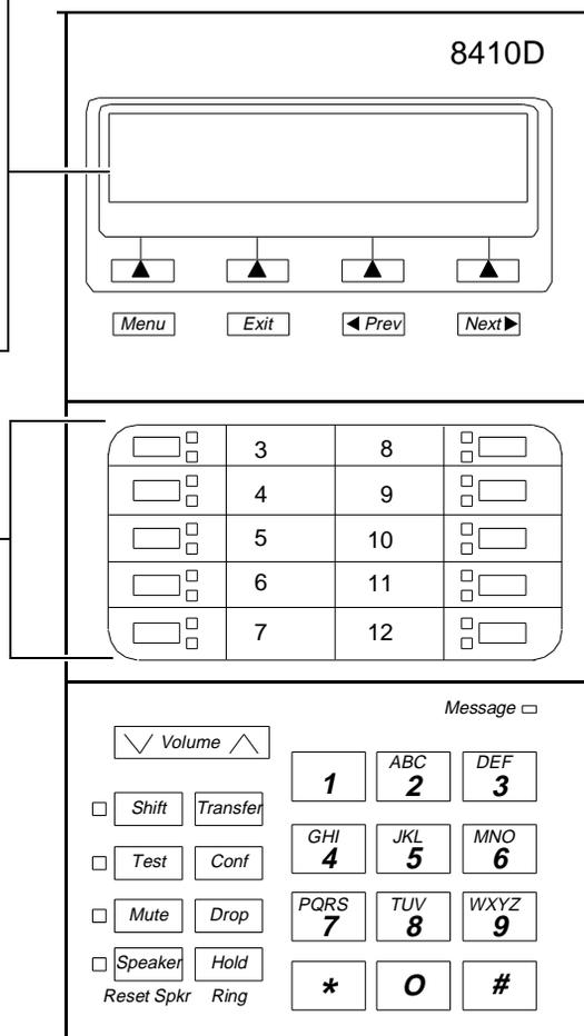
**Figure 12-10. Button Numbering for Administering the 8410 Voice Terminal Connected to a System 85 or a DEFINITY G2**
