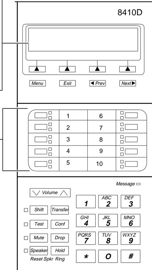
**Figure 12-9. Button Numbering for Administering the 8410 Voice Terminal Connected to a System 75, a DEFINITY G1 or G3, or a DEFINITY ECS**
