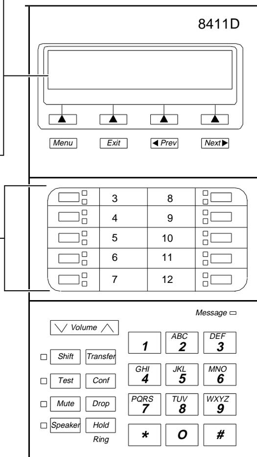
**Figure 12-15. Button Numbering for Administering the 8411 Voice Terminal Connected to a System 85 or a DEFINITY G2**
