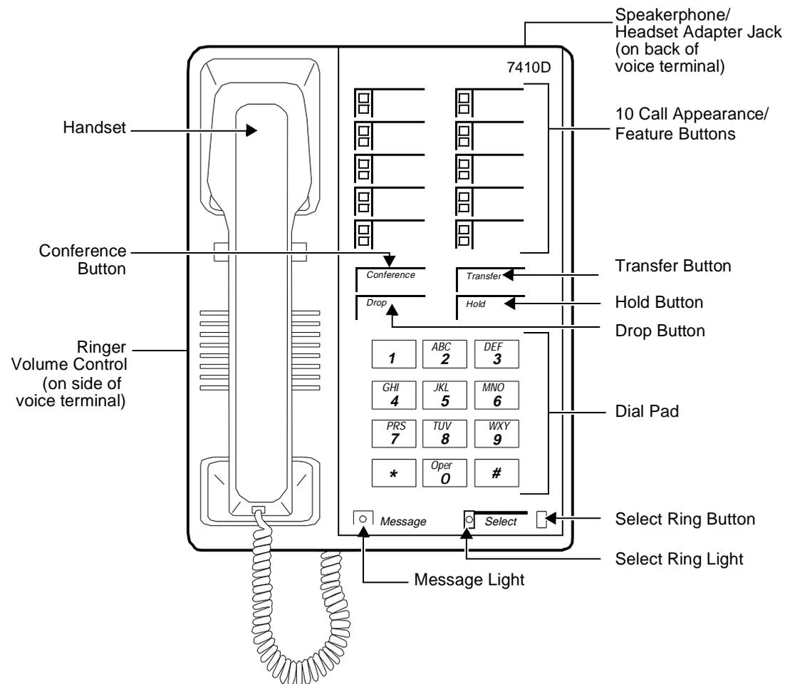
Figure 11-26. The 7410D (7401D01A) Voice Terminal
