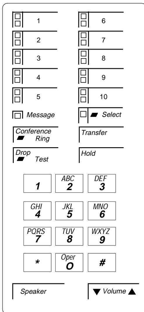
Figure 11-30. Button Numbering for Administering the 7410 Plus Voice Terminal Connected to a System 75, a DEFINITY G1 or G3, or a DEFINITY ECS
