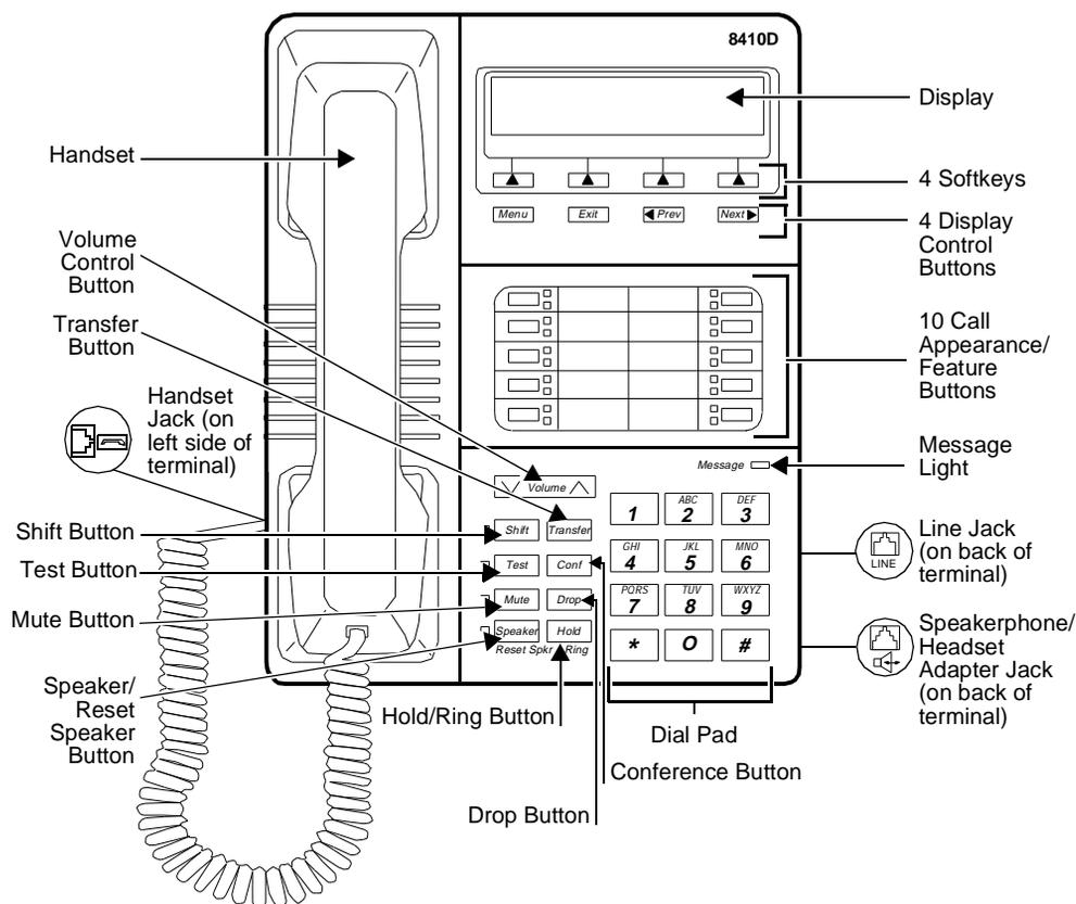
**Figure 12-8. The 8410D Voice Terminal (with Display)**
