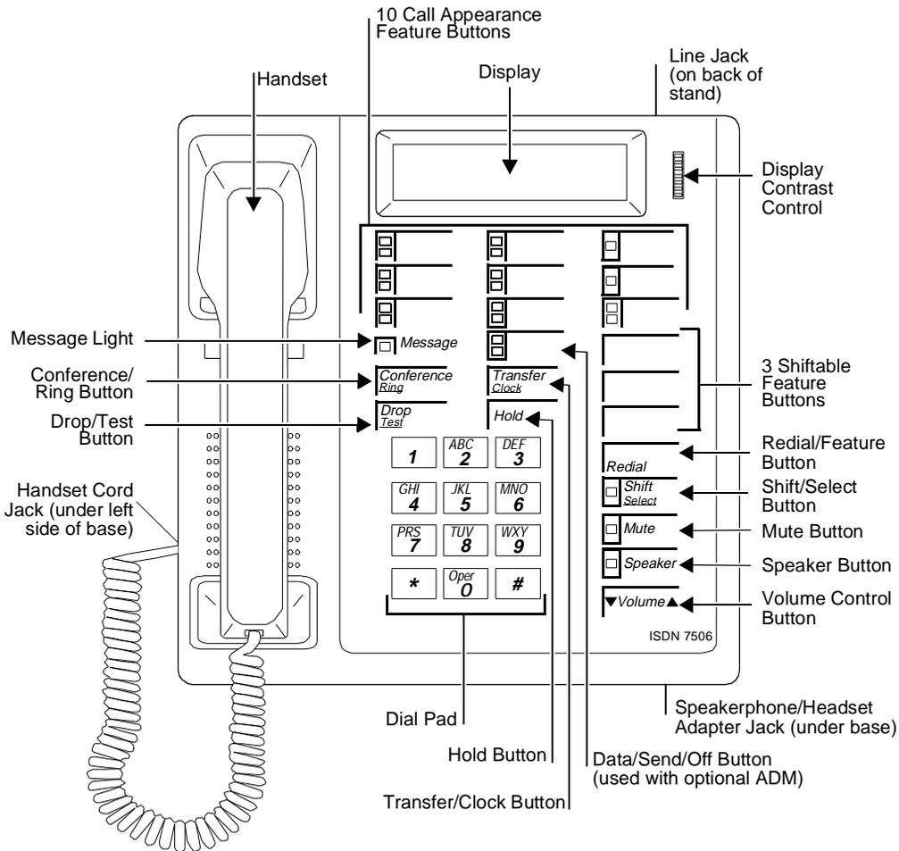
Figure 16-2. The 7506 Asynchronous Data Modular Display Terminal
