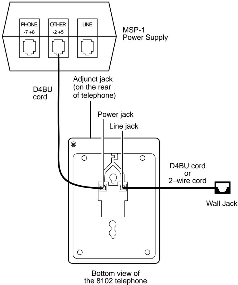
**Figure 5-3. Local Powering Arrangement for Adjuncts Connected to the 8102 Analog Telephone**
