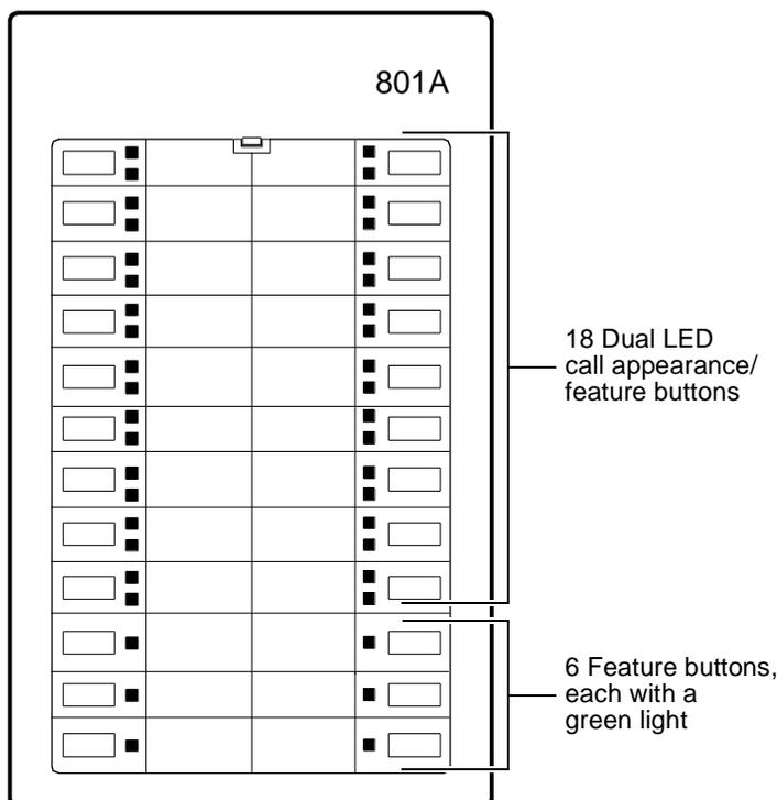
**Figure 19-4. The 801A Expansion Module**
