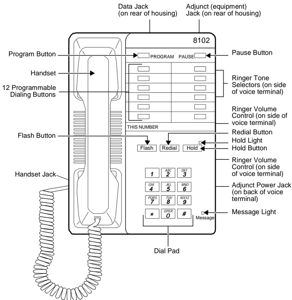
**Figure 15-3. The 8102 and 8102M Telephone**
