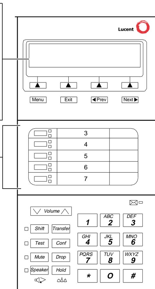
Figure 12-7. Button Numbering for Administering the 8405 Voice Terminal Connected to a System 85 or a DEFINITY G2
