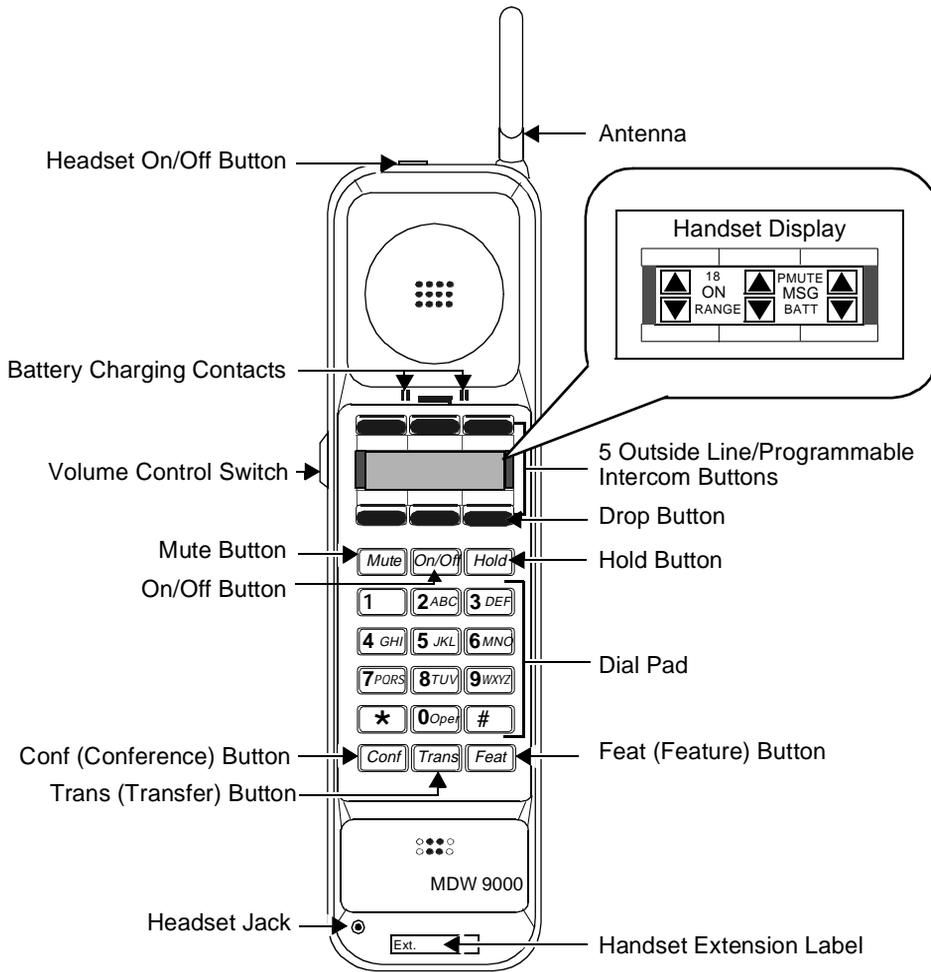
Figure 17-5. The MDW 9000 Telephone, Including Enlarged Display Area
