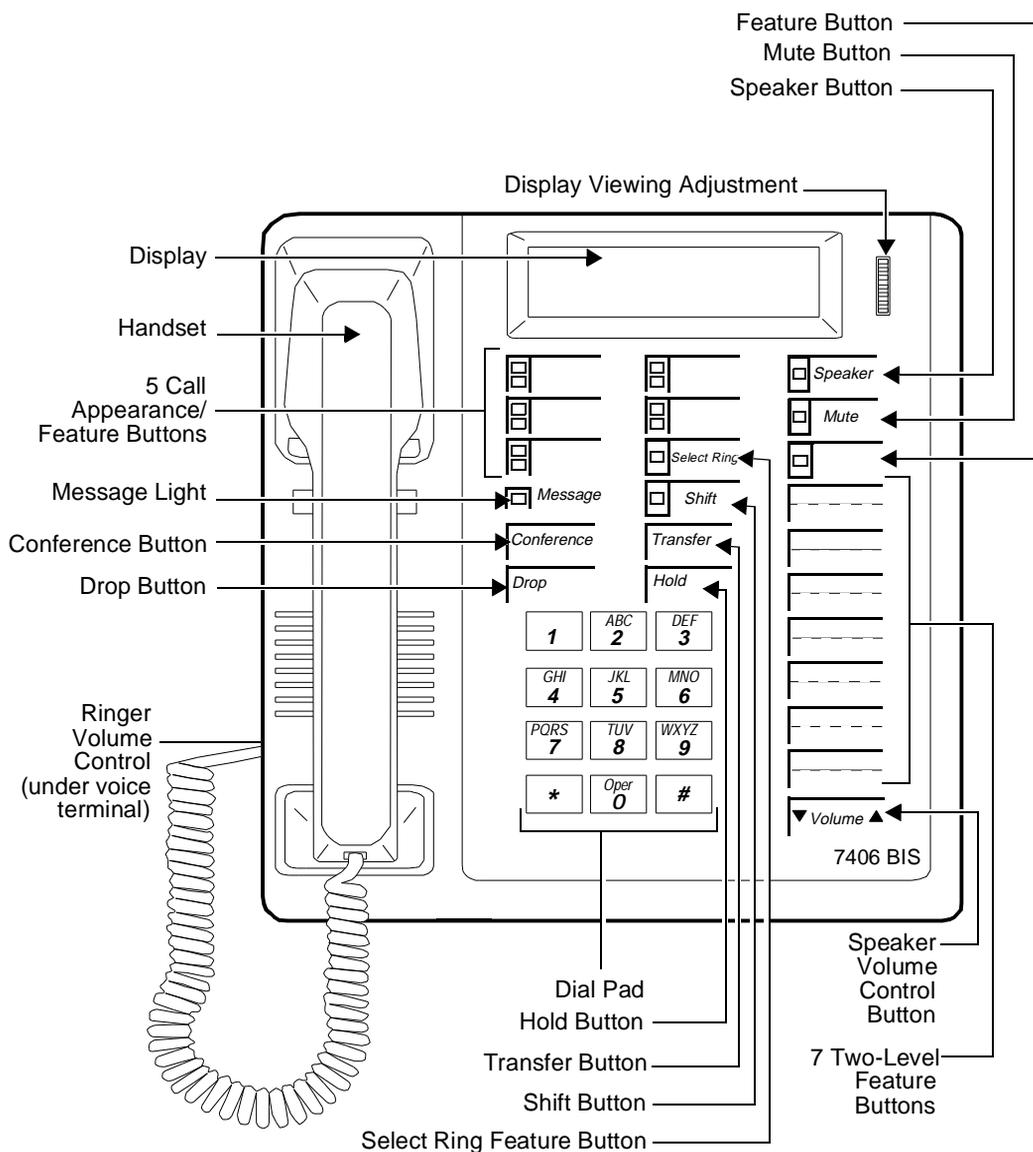
Figure 11-11. The 7406BIS (7406D05A) Voice Terminal with Display
