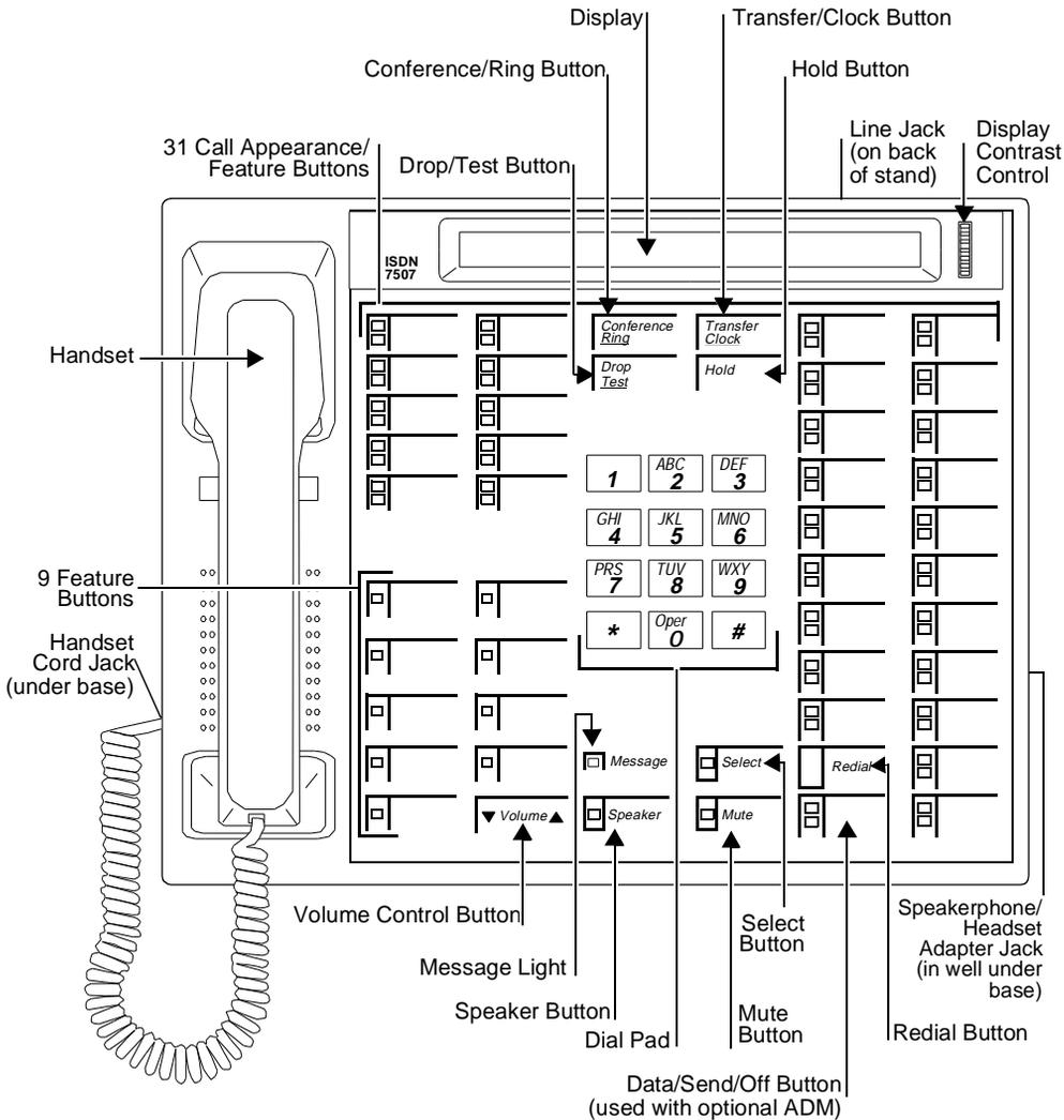
**Figure 16-3. The 7507 Asynchronous Data Modular Display Terminal**
