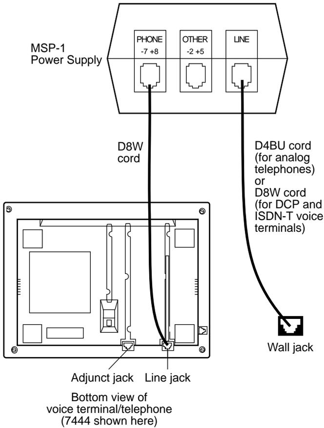
**Figure 5-2. Local Powering Arrangement for: ISDN-T Voice Terminals; the DCP 7444 and 8434/8434DX Voice Terminals (for their VF Displays); and Adjuncts Connected to All Telephones Except the 8102**
